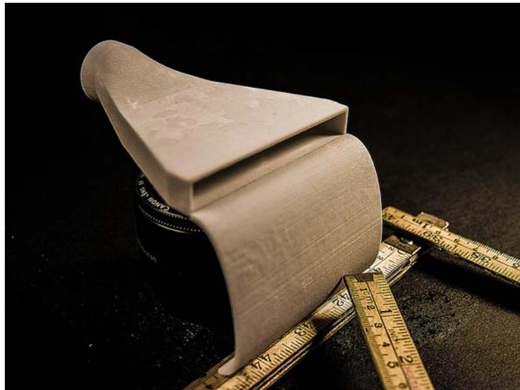
*Figure 22 3D printed prototype of local extractor.*
