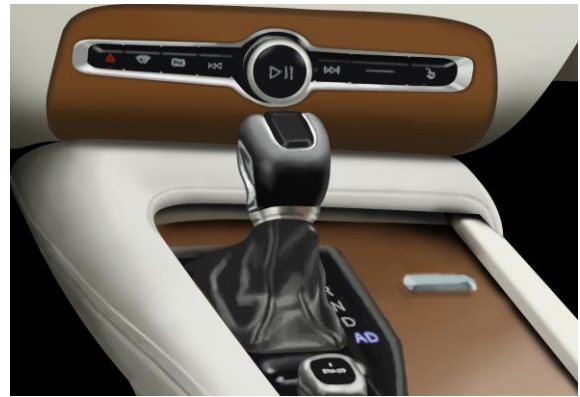
Figure 42 - Above the AD mode is active and the vehicle is operating the driving task itself on an AD-certified road (level 3 NHTSA).
