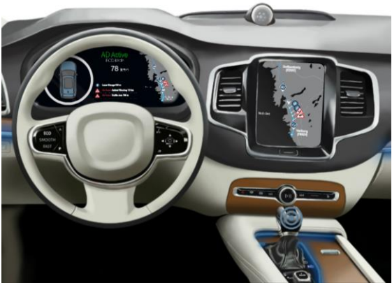
Figure 54 – Touch point on the gearshift showing the interactive map on the CSD.
