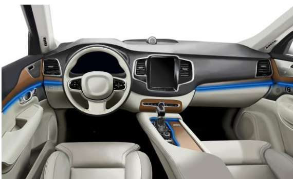
Figure 44 - Interior in AD mode with blue ambient light.
