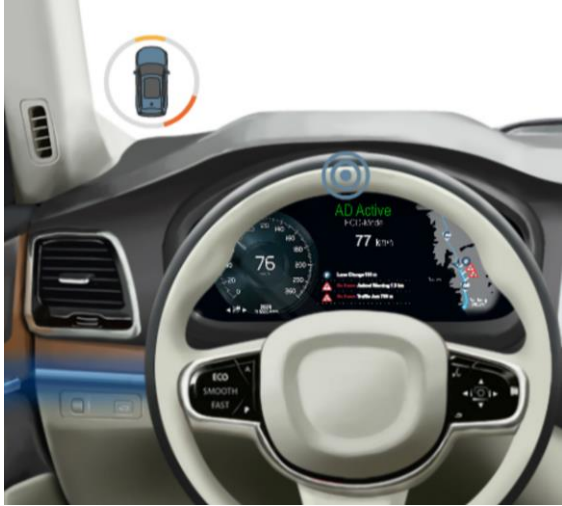
Figure 55 – Touch point on the steering wheel moving the ring concept to the HUD and a speedometer will appear instead in the DIM.
