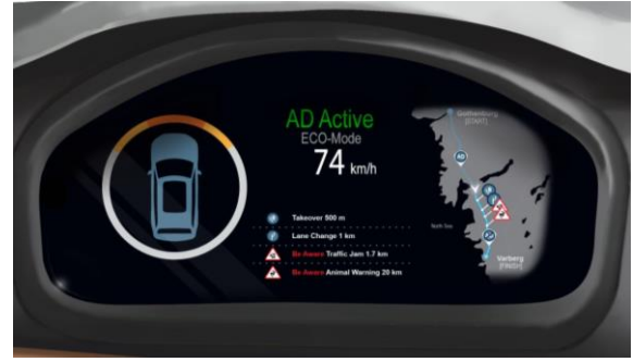
Figure 48 - DIM in AD mode showing interactive map and object recognition system.
