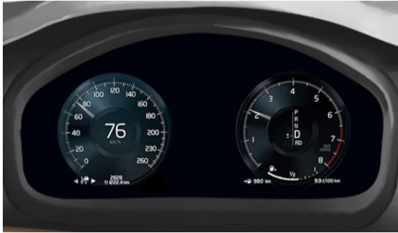
Figure 47 - DIM in manual mode showing gauges.
