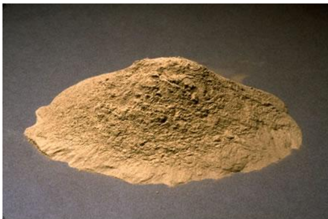
Figure 1.3-1: Fly ash powder, as a mineral product from industrial coal combustion.
