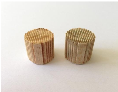
Figure 3.3: Photograph of monolith samples after ash coverage by washcoating.
