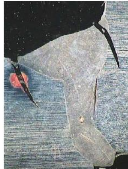
Figure 2.32 Fatigue test a) Fatigue test arrangement b) Crack pattern in specimen (Alam et al. 2009).
