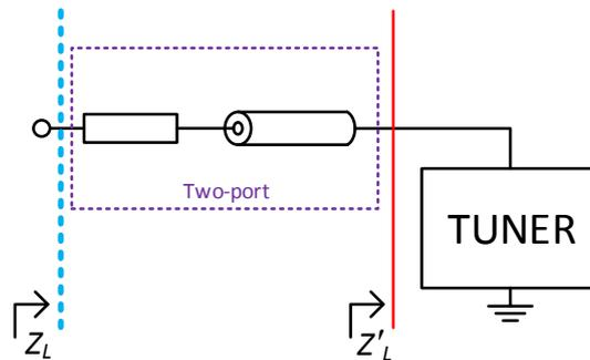
**Figure 2.11:** Output impedance de-embedding. The output transmission lines (microstrip and fixture connector) can be merged into one two-port terminated by the tuner.
