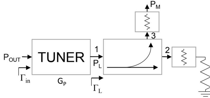
**Figure 2.13:** Tuner and coupler on the output side.
