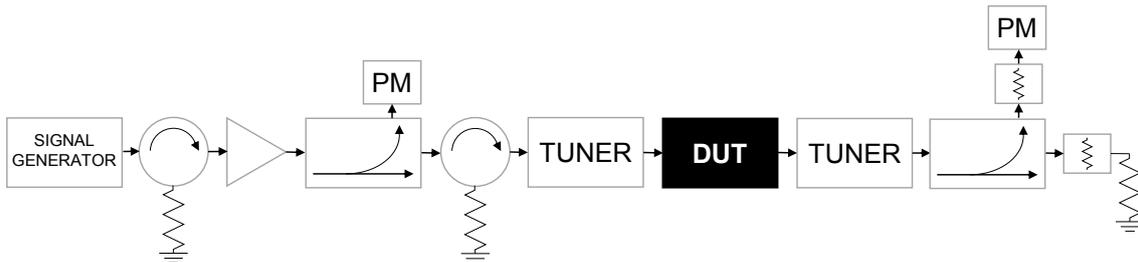
**Figure 2.9:** Characterization setup for load-pull and source-pull measurements.
