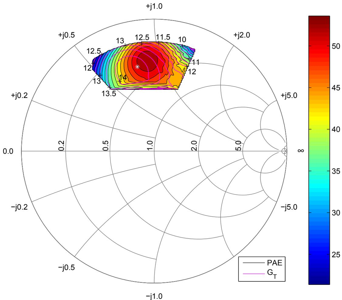
**Figure 3.3:** Load-pull at high power for the main amplifier. The PAE contour interval is 2 percentage points.
