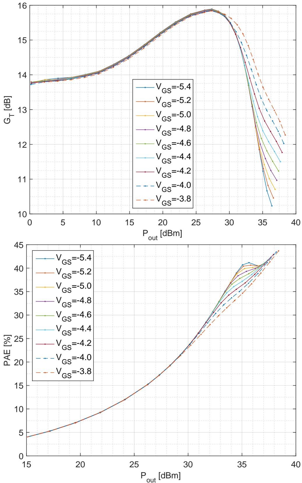
**Figure 5.3:** Measured transducer gain and power added efficiency results versus output power at 6 GHz for different **aux.** gate bias values.  $V_{DS} = 40$  V and  $V_{GSmain} = -2.84$  V.
