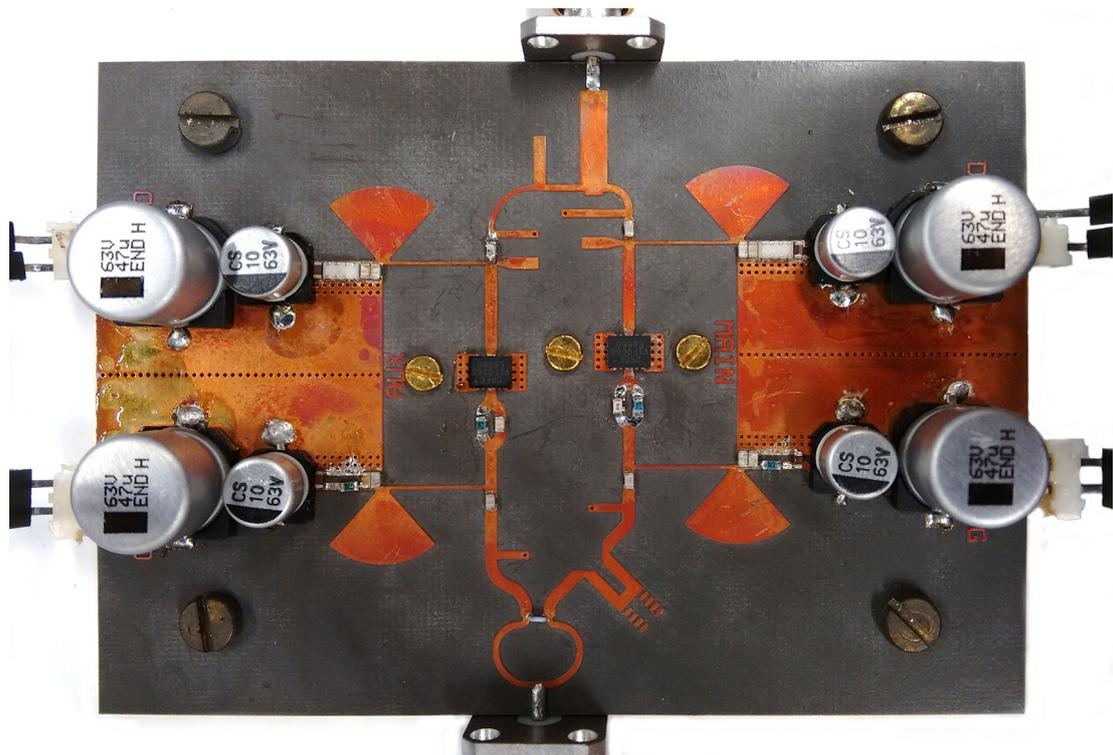
**Figure 5.1:** Assembled 6 GHz Doherty PA prototype developed from load-pull measurement data. PCB dimension are 61x86 mm.
