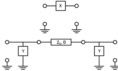
**Figure 4.9:** The upper network, a series inductance, will be replaced by the lower network, which is realizable using only transmission lines.
