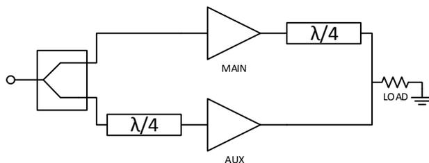
**Figure 2.1:** Block diagram of a classical DPA [6] in its simplest form.
