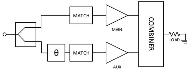
**Figure 2.3:** Block diagram of the Doherty PA design approach [11] used in this work.
