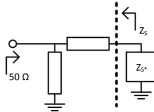
**Figure 4.4:** Matching network topology for the transistors.
