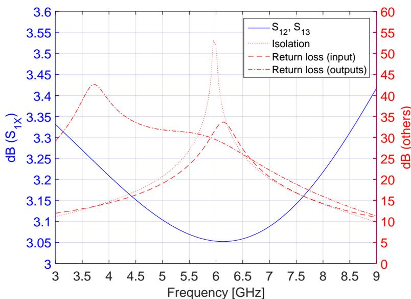
**Figure 4.3:** Simulated performance of the input power splitter, after optimization.
