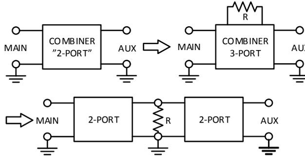
**Figure 4.6:** Combiner design process, going from a lossy two-port representation of the output combiner to equivalent lossless two-ports terminated by the load. Later, the latter is realized using microstrips.
