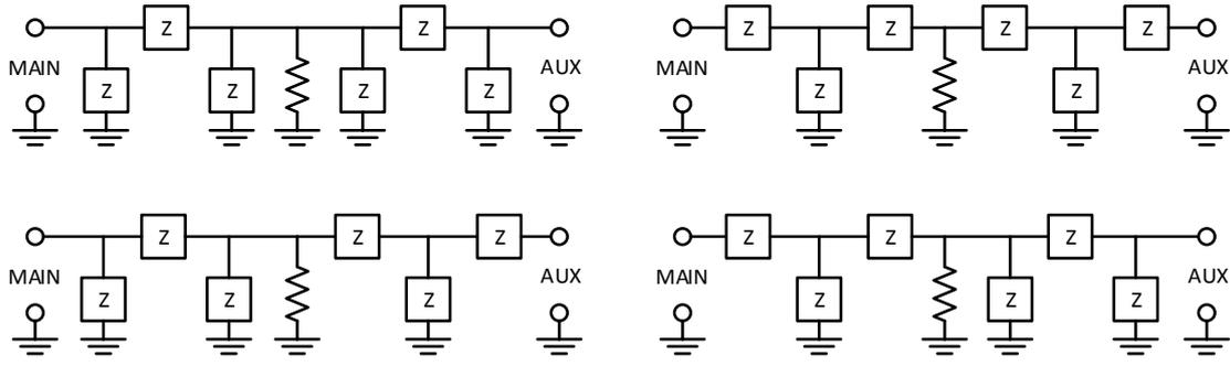
**Figure 4.7:** The four different combiner topologies. The symbols are used to represent impedances; they are not necessarily of the same value.
