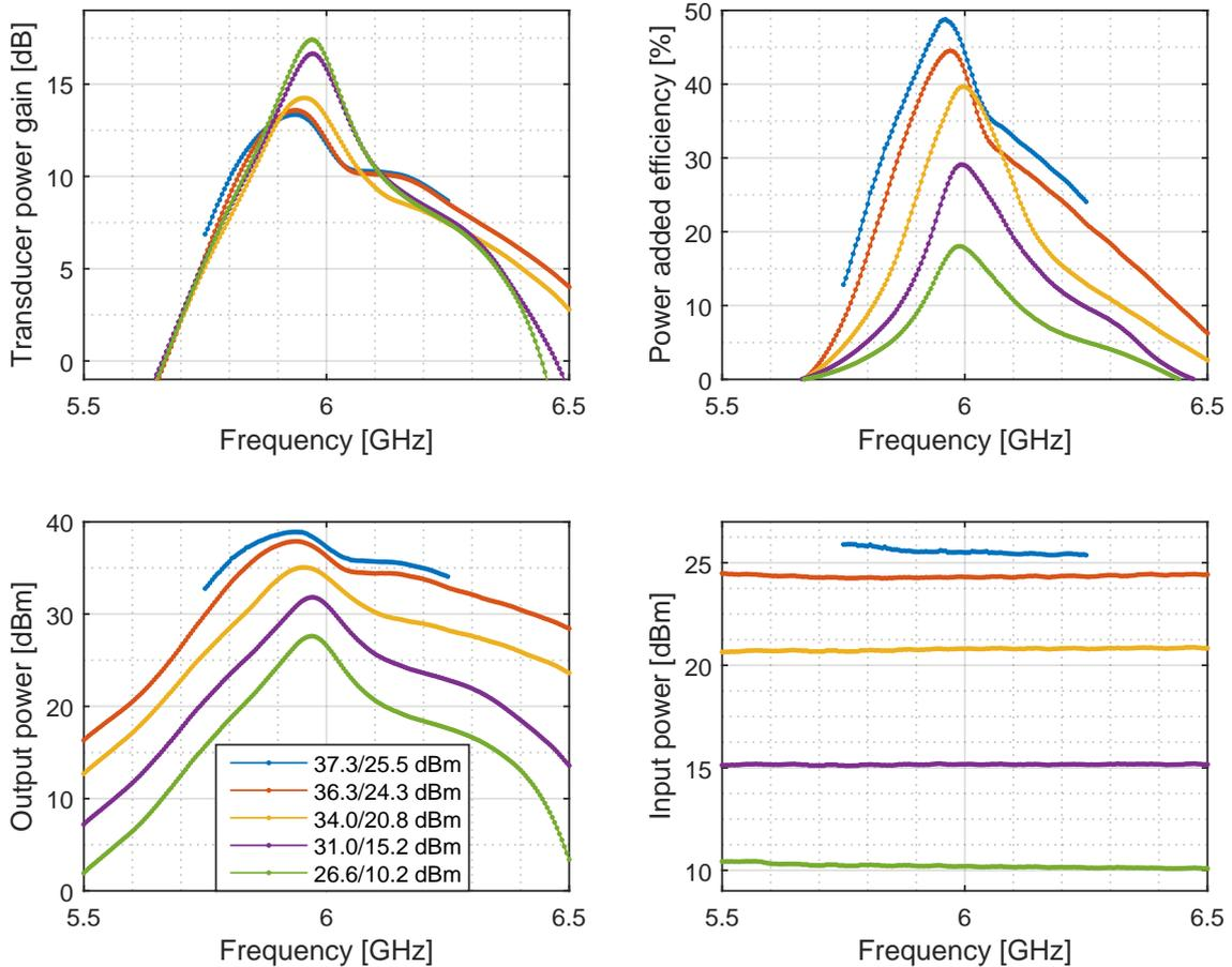
**Figure 5.6:** Frequency sweeps for a selection of power levels. The legend entries give the output and input powers at the center frequency.  $V_{DS} = 40$  V,  $V_{GS_{main}} = -2.85$  V,  $V_{GS_{aux}} = -4.5$  V.
