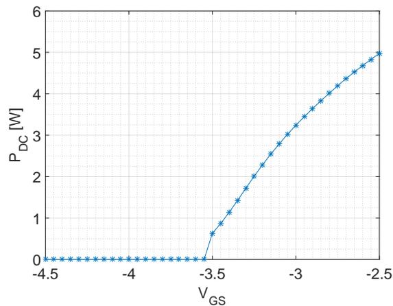
**Figure 3.2:** DC power consumption for a fixed input power level while sweeping  $V_{GS}$ , for finding the point at which the amplifier shuts off.
