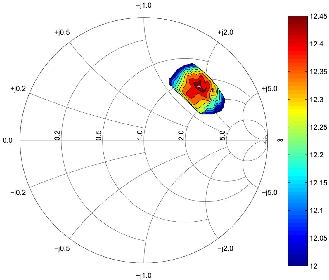
**Figure 3.7:** Source-pull results for class C biasing. The transducer power gain is plotted when the true input power was between 23.00 dBm and 23.33 dBm.
