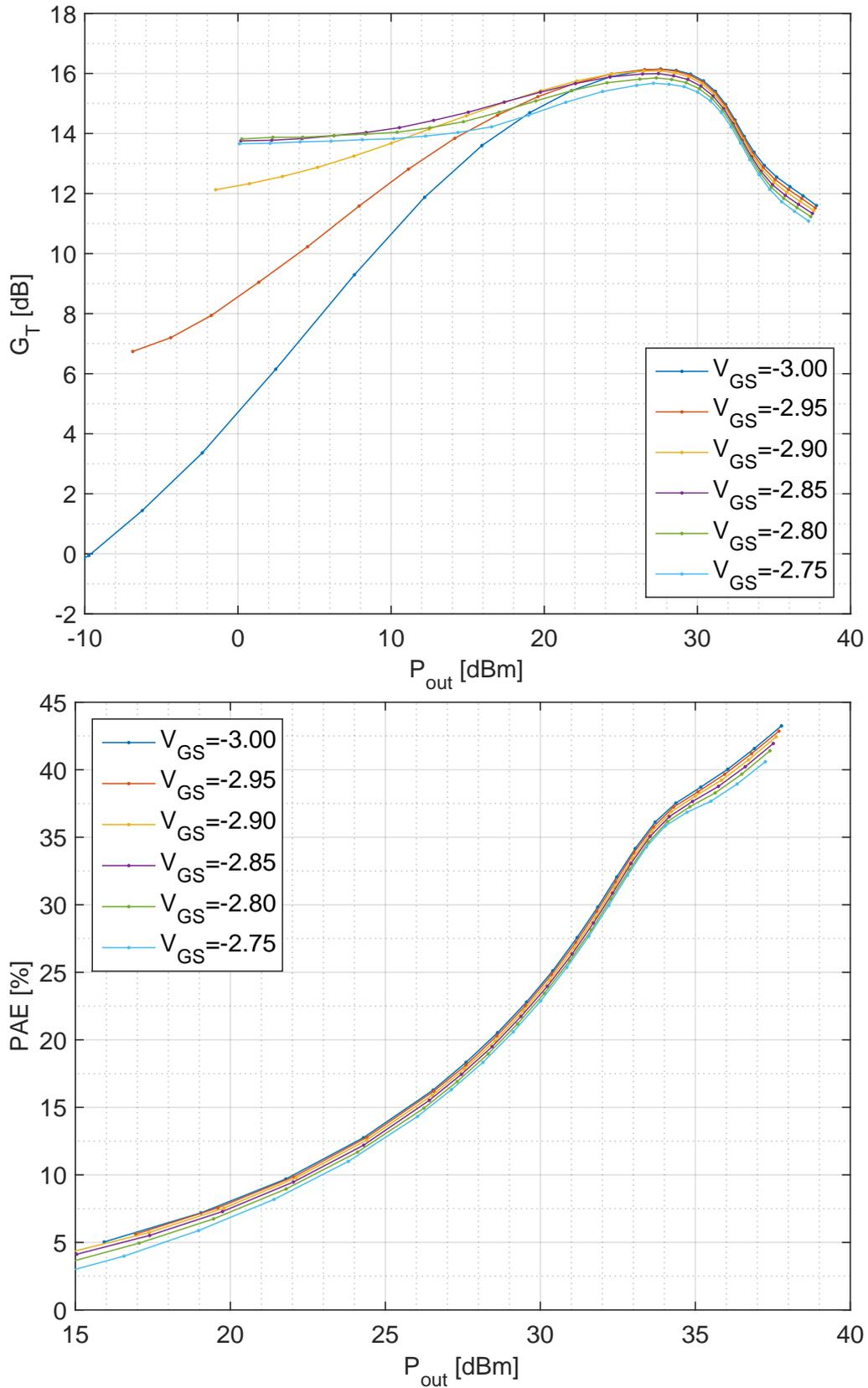
**Figure 5.4:** Measured transducer gain and power added efficiency results versus output power at 6 GHz for different **main** gate bias values.  $V_{DS} = 40$  V and  $V_{GSaux} = -4.5$  V.
