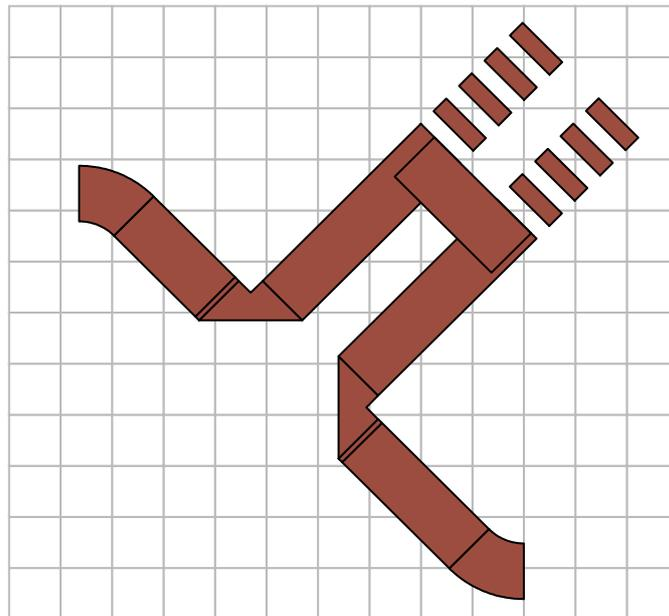
**Figure 4.13:** Trimmable phase shifter for the DPA. Grid size 1x1 mm.
