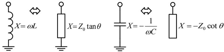
**Figure 4.8:** Reactive shunt elements can easily be replaced by stubs.
