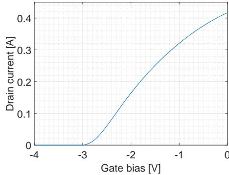
**Figure 2.4:** Simulated DC characteristics of the transistor. Drain current versus gate bias voltage at  $V_{DS} = 40$  V.
