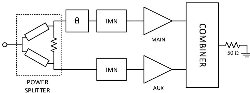
**Figure 4.1:** Block view of complete amplifier. IMN stands for input matching network.  $\theta$  represents the phase shifter.
