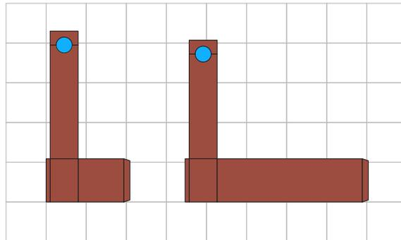
**Figure 4.5:** Input matching networks for the main amplifier (left) and the auxiliary amplifier (right). The left side of each network is the  $50 \Omega$  input. Grid size  $1 \times 1 \text{ mm}$ .
