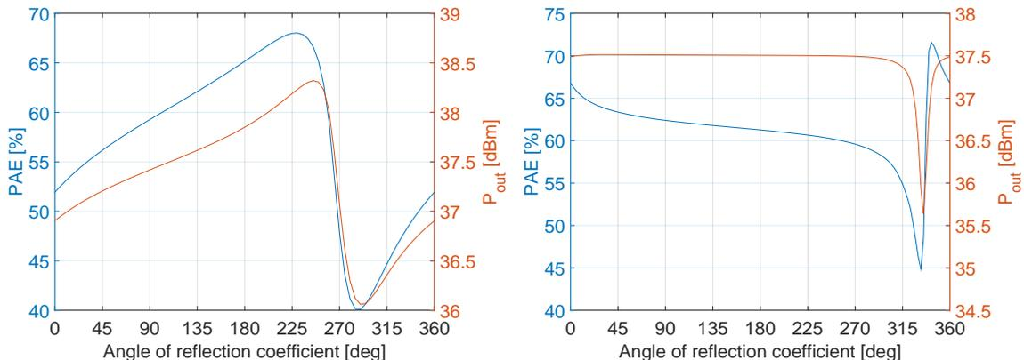
**Figure 2.7:** Sweep of the phase of the second harmonic termination for the load (left) and source (right). The input power was 21 dBm.
