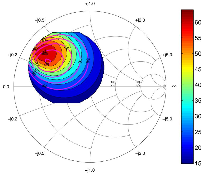
**Figure 2.6:** Simulated load-pull of the transistor at 6 GHz with 21 dBm of input power. The color bar indicates PAE in percentage and the violet lines show delivered power contours in dBm.
