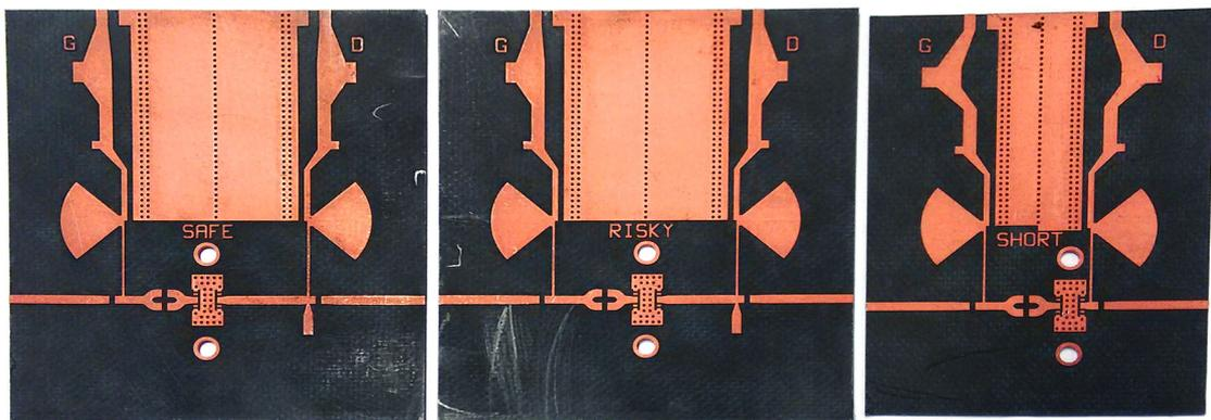
**Figure 2.8:** The three test boards before assembly. (The non-straight appearance of the edges, especially visible in the right board, is just a result of lens distortion).
