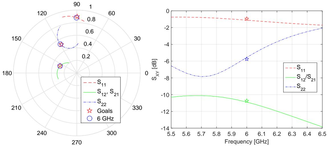
**Figure 4.12:** Combiner S-parameter simulation results between 5.5–6.5 GHz. Left: comparison of achieved values at the center frequency (circles) with targeted values (stars). Right: S-parameters in dB compared with the target values at 6 GHz.
