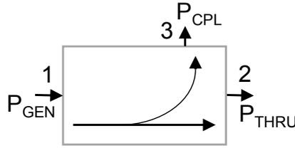
**Figure 2.12:** Directional coupler at input.
