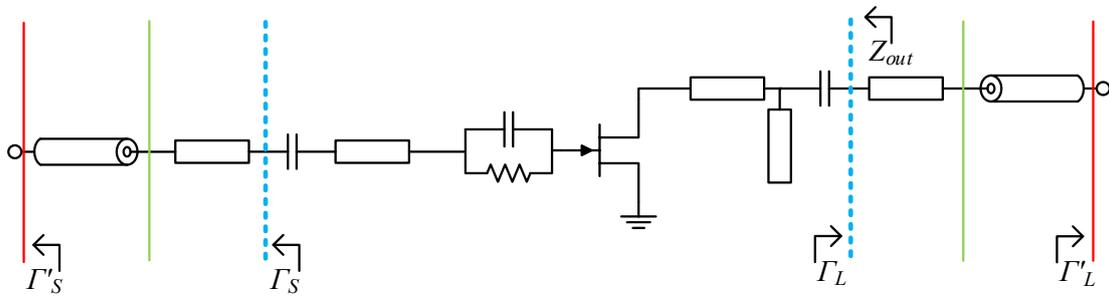
**Figure 2.10:** Simplified schematic and desired reference planes drawn as dashed blue lines (DUT plane). The red lines show the impedance measurement reference plane. The solid green lines represent the extent of the circuit board.
