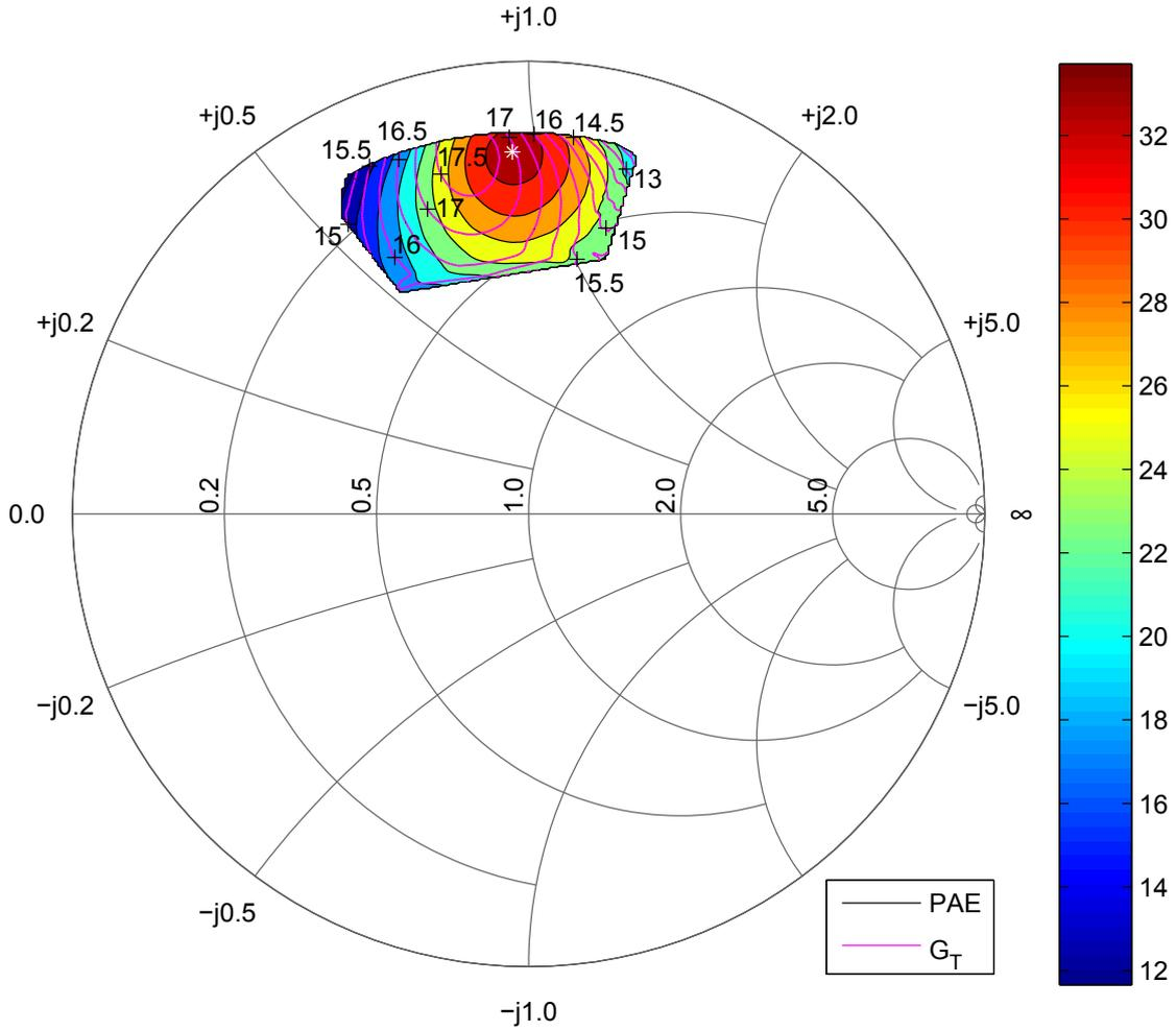
**Figure 3.4:** Load-pull at back-off for the main amplifier. The PAE contour interval is 2.5 percentage points.
