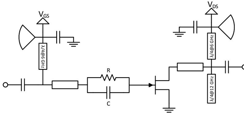
**Figure 2.5:** Simplified schematic of the test circuit for load-pull measurements. The characterization not only includes the transistor, but the whole amplifier unit including bias lines, stability network and coupling capacitors.
