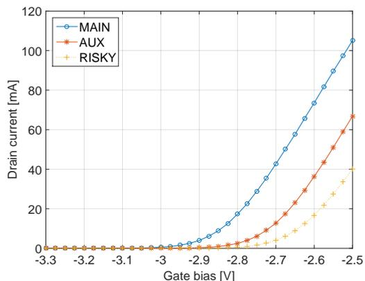
**Figure 5.2:** Gate bias sweeps of the transistors on the final DPA, with previous sample as comparison.  $V_{DS} = 40\text{ V}$ .
