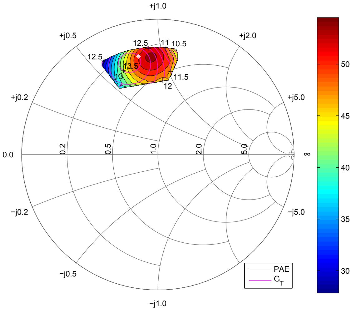
**Figure 3.5:** Load-pull with class C biasing, for the auxiliary amplifier. The PAE contour interval is 2 percentage points.
