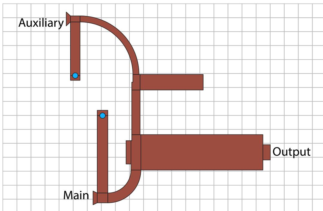
**Figure 4.11:** Layout of the final output combiner for the 6 GHz DPA, including the quarter wave transformer for  $50\Omega$  output. Outer dimensions 14.5x13.8mm, grid size 1x1 mm.
