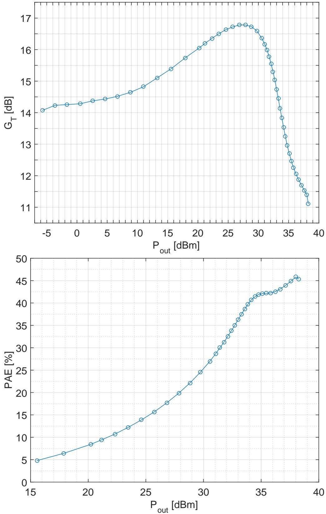
**Figure 5.5:** Final power sweeps of the DPA at 6 GHz.  $V_{DS} = 40$  V,  $V_{GSmain} = -2.85$  V,  $V_{GSaux} = -4.5$  V.
