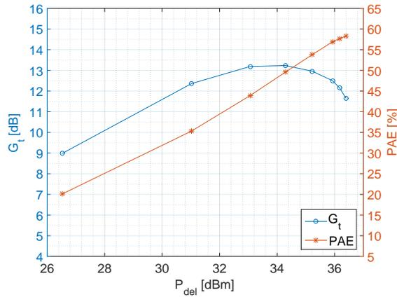
**Figure 3.9:** Power sweep for class C. Note that the scales are different. When the power level is decreased further, the device soon shuts off.
