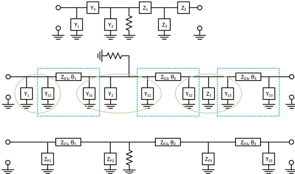
**Figure 4.10:** Illustration of the conversion process from lumped element network to transmission line network. The dotted rectangles outline the replaced series elements, and the ovals outline elements suitable for parallel combination. The Z-blocks and Y-blocks are used to represent impedances/admittances, they are not all identical. The same applies to the transmission lines.
