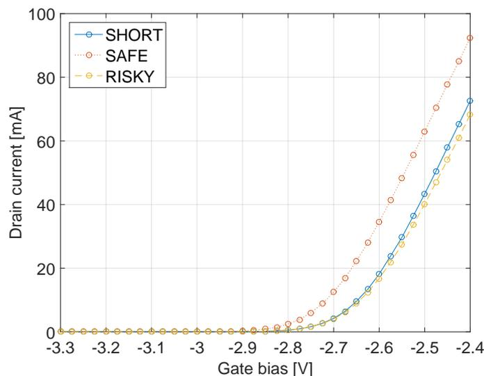
**Figure 3.1:** Bias sweeps of the three transistors used on the test boards.
