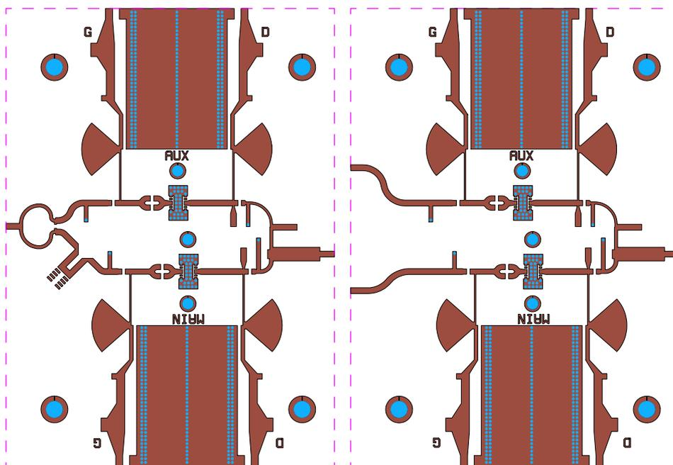
**Figure 4.14:** Final PCB layouts, natural size (on A4 paper). The outer dimensions of a board is 61x86 mm.
