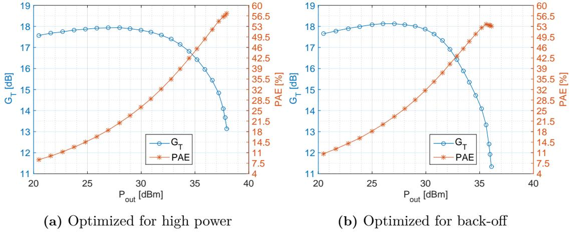
**Figure 3.8:** Power sweeps using approximately final load and source impedances for class B.
