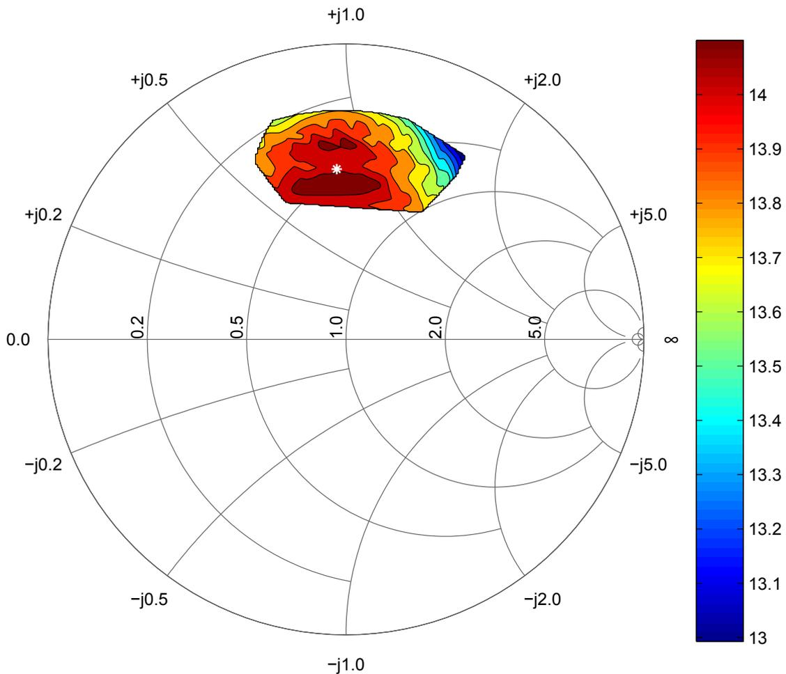
**Figure 3.6:** Source-pull results for class B biasing. The transducer power gain is plotted when the true input power was between  $23.00 \text{ dBm}$  and  $23.35 \text{ dBm}$ .
