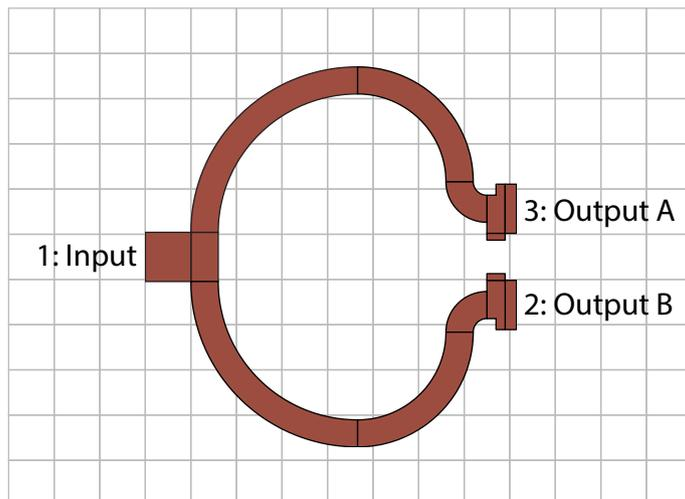
**Figure 4.2:** Equal-split Wilkinson power divider geometry. Outer dimensions of splitter 7.2x8.4 mm, grid size 1x1 mm.
