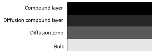
Figure 5 Schematic structure of a nitrided layer.
