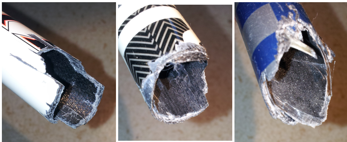
Figure 1.2: Samples of broken floorball sticks
