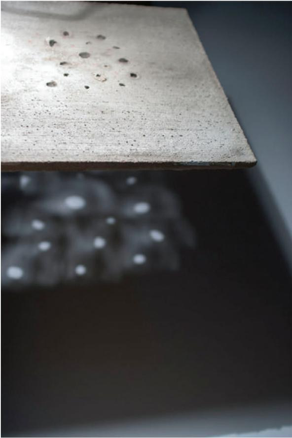
*Model test of openings in concrete shell, with different light angles*
