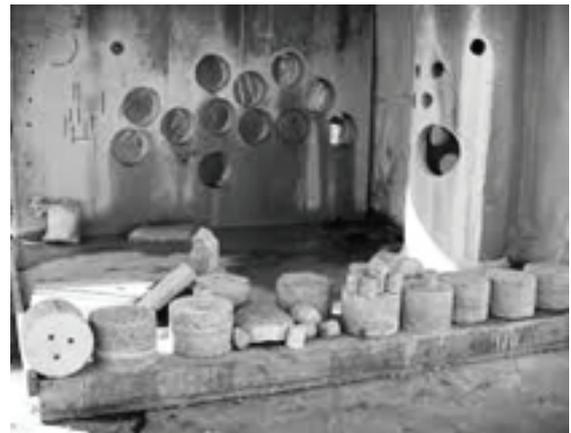
Core drilling is a common method to make holes in existing concrete structures.
