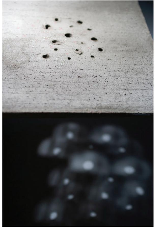
*Model test of openings in concrete shell, the light and shadow play alters with the angle*
