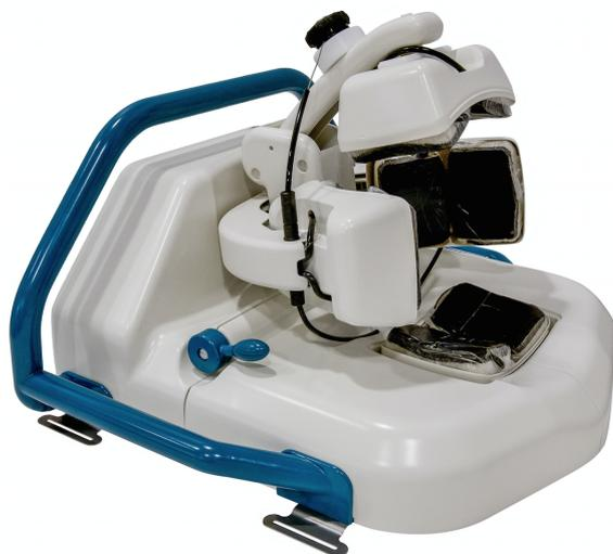
Figure 1: A picture of Strokefinder MD100. It's a headrest stroke diagnostic instrument where measurements are performed in a supine position by eight broadband microwave antennas with various combination of channels.
