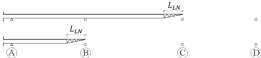
Figure 4.25 Launching stages considered.
