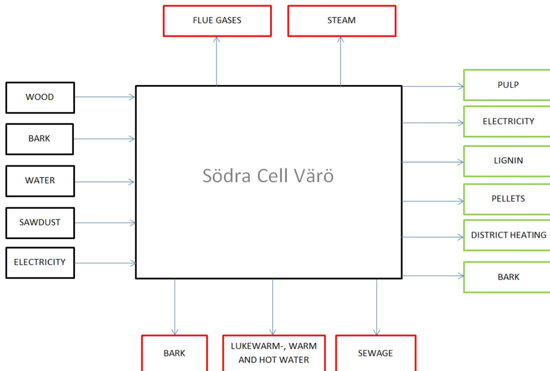
Figure 3. A schematic picture of the system boundaries of this master thesis. The black boxes are input products into the system, the green boxes indicate products that potentially can be sold on the market and the red boxes indicate potential system losses.
