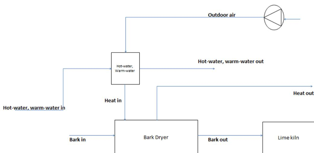
Figure 17. Schematic picture of the modelled bark dryer.
