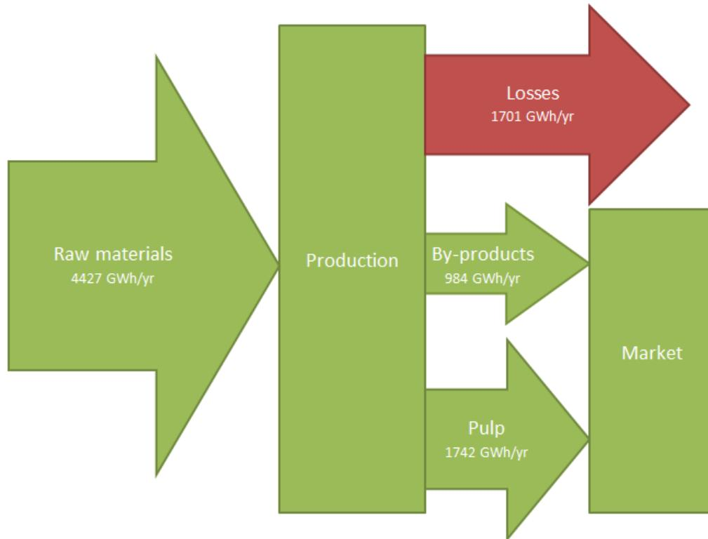
Figure 2. Schematic picture of the energy balance at Södra Cell Värö. (Rudén, 2014, Morin, 2014)
