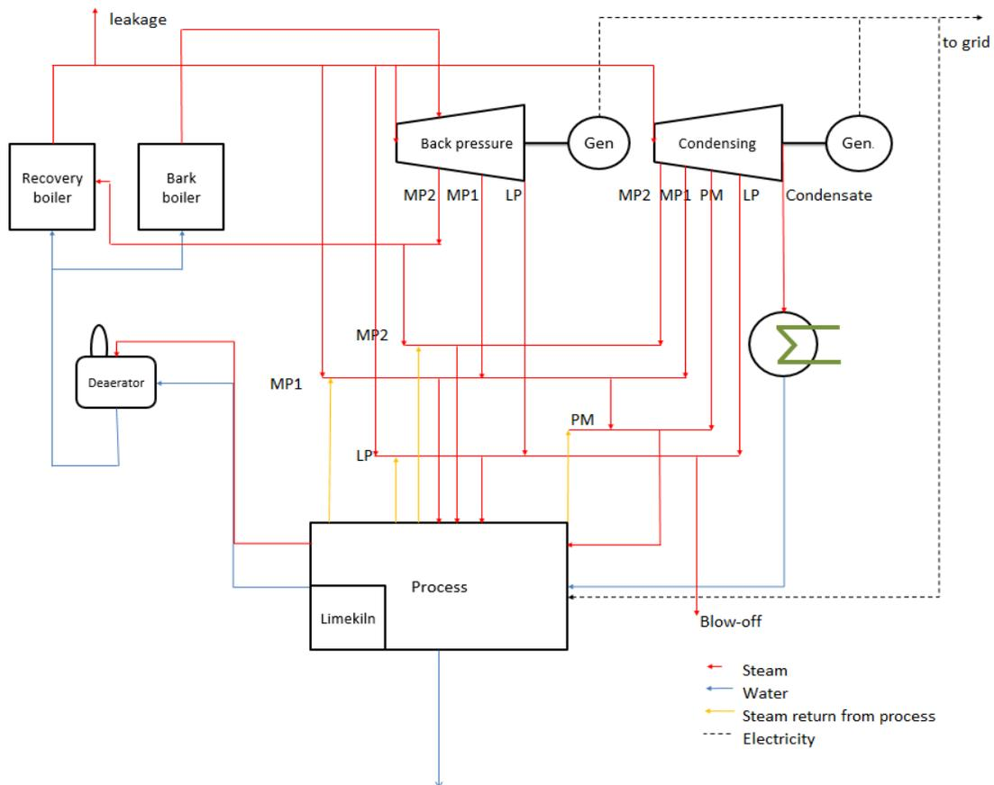
Figure 9. A simplified schematic picture of the steam system for the base case.
