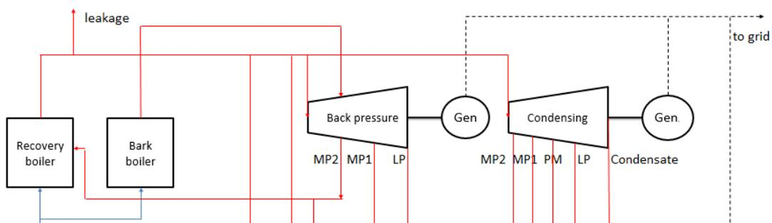
Figure 11. Schematic picture of the parts of the system used in Scenario 1: Bark Burning.
