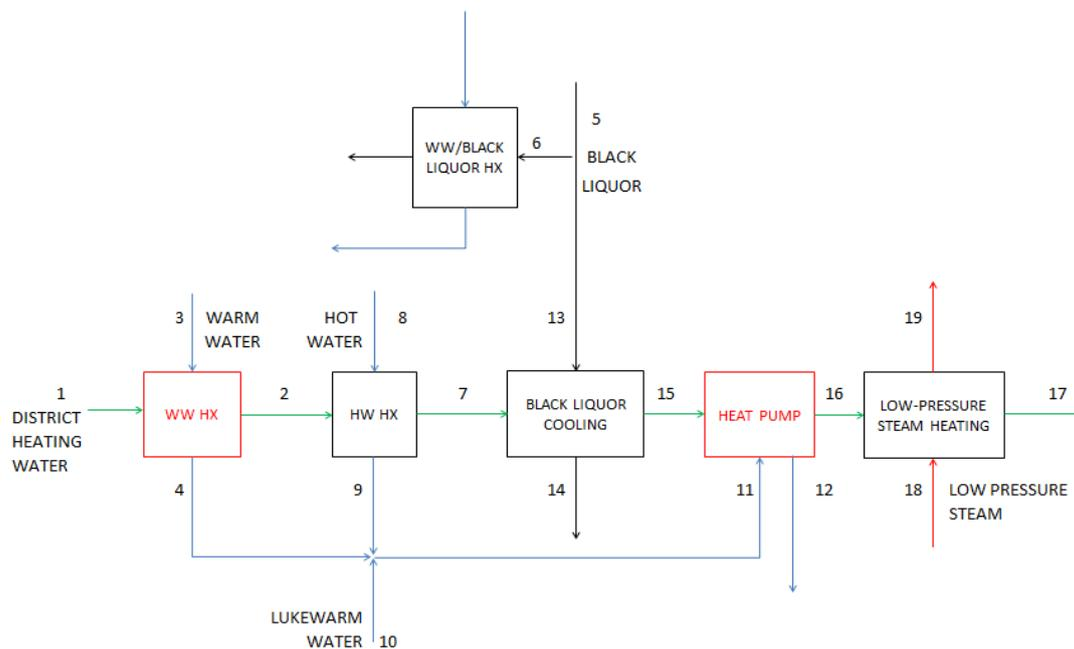
Figure 14. Schematic picture of the heat exchanger network for Scenario 3c: Increased district heating capacity to Varberg by implementing a warm water heat exchanger and a heat pump.
