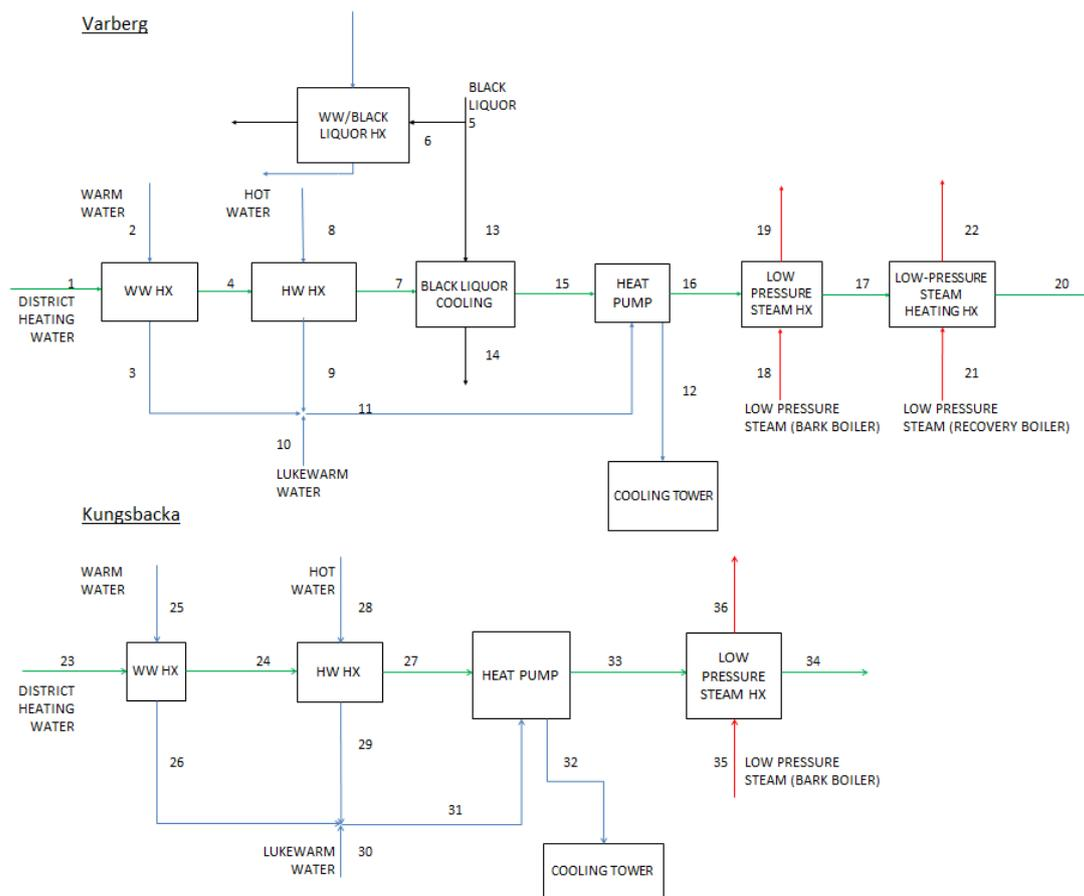
Figure 16. Schematic picture of the heat exchanger network for Scenario 3e: Maximum district heating capacity to Varberg and deliveries to Kungsbacka.
