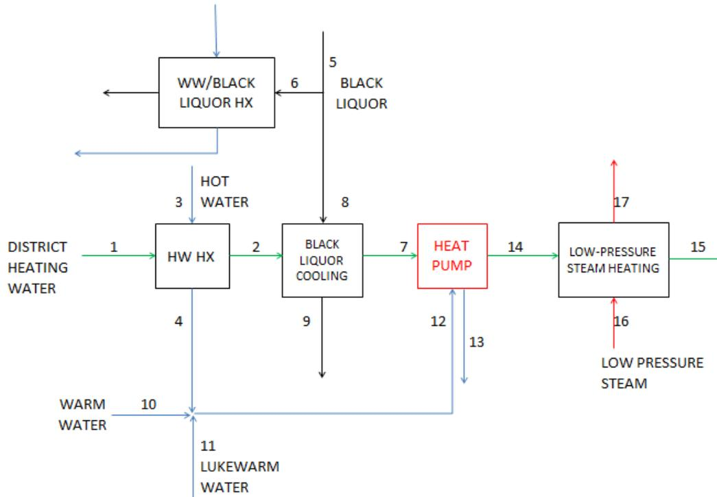
Figure 13. Schematic picture of the heat exchanger network for Scenario 3b: Increased district heating capacity to Varberg by implementing a heat pump.
