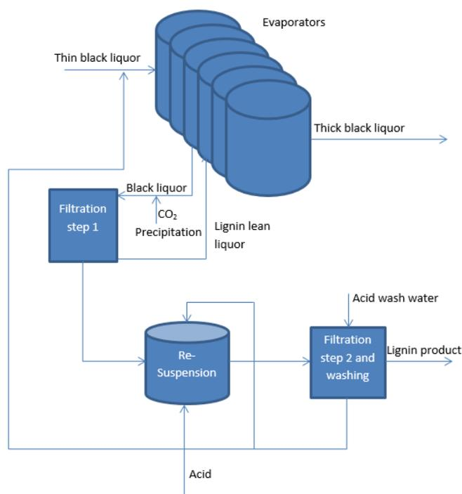
Figure 7. Schematic overview of the LignoBoost process for lignin extraction.
