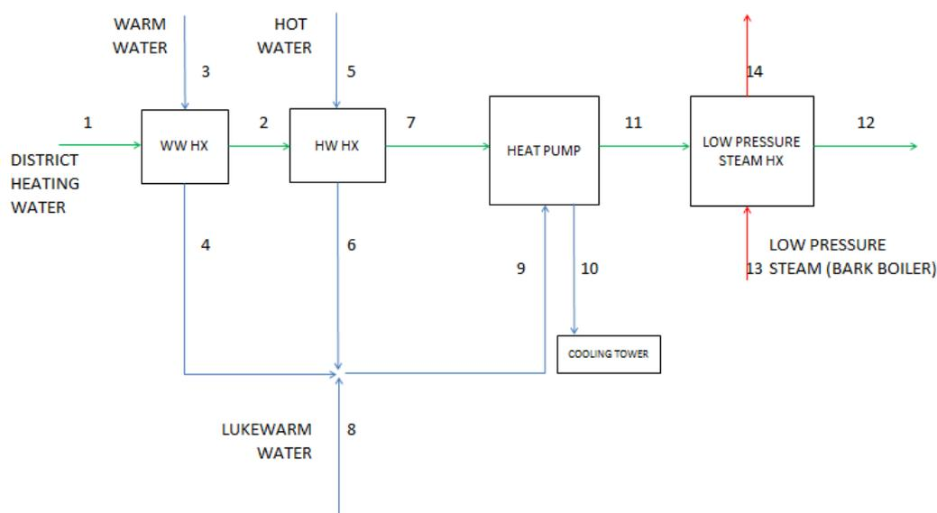
Figure 15. Schematic picture of the heat exchanger network for Scenario 3d: Expanding the district heating network to Kungsbacka while maintaining planned deliveries to Varberg. The figure only shows the heat exchanger network to Kungsbacka, however the Varberg heat exchanger network is the same as in Figure 10.
