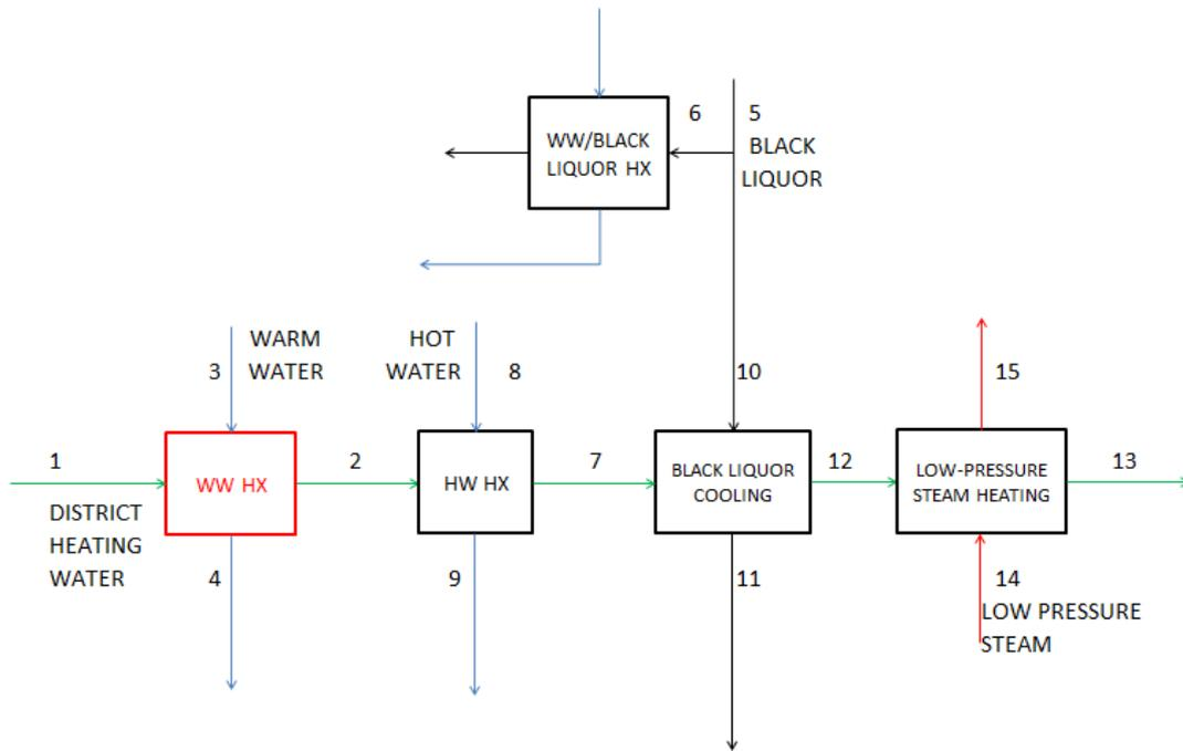
Figure 12. Schematic picture of the heat exchanger network for Scenario 3a: Increased district heating capacity to Varberg by implementing a warm water heat exchanger.
