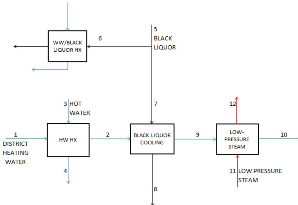
Figure 10. Schematic picture of the heat exchanger network for the planned district heating system.
