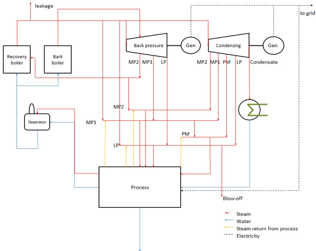
**Figure 5. The energy system of the Södra Cell Värö pulp mill.**
