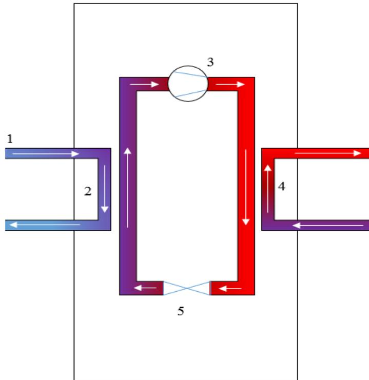
**Figure 30. Schematic picture of a heat pump.**
