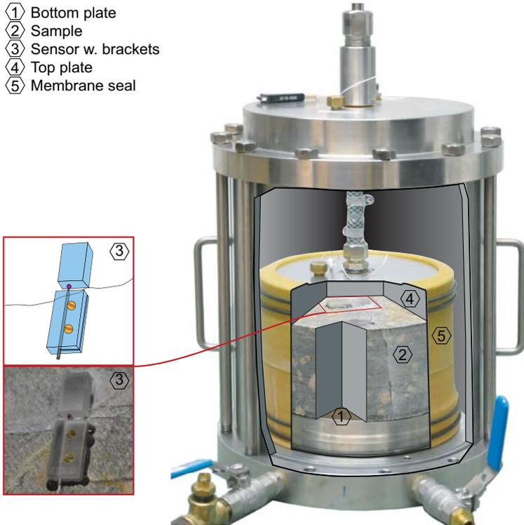
Figure 14: Cutaway view of the HM permeameter with a sample mounted. (Modified from Publication V)
