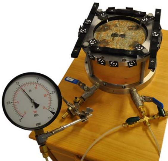
Figure 17: The permeameter, modified to enable the surface scanning and referencing procedure. A fractured sample is confined to 1.0 MPa inside, ready for the first step of the surface scanning procedure. (Figure from Publications VI and VII).
