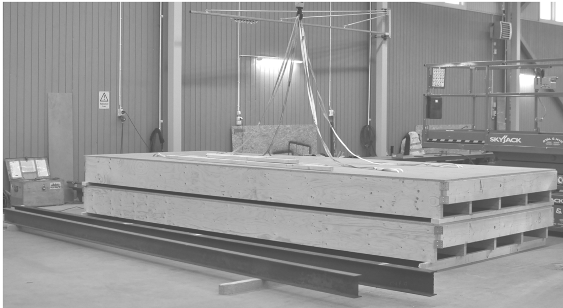
Figur0.1 Testing site with the two test specimens and the steel I-beams used for the boundary conditions.
