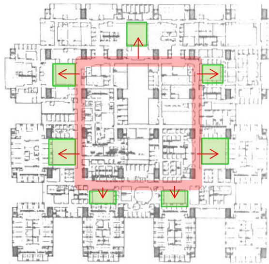
Main corridor links to all courtyards
