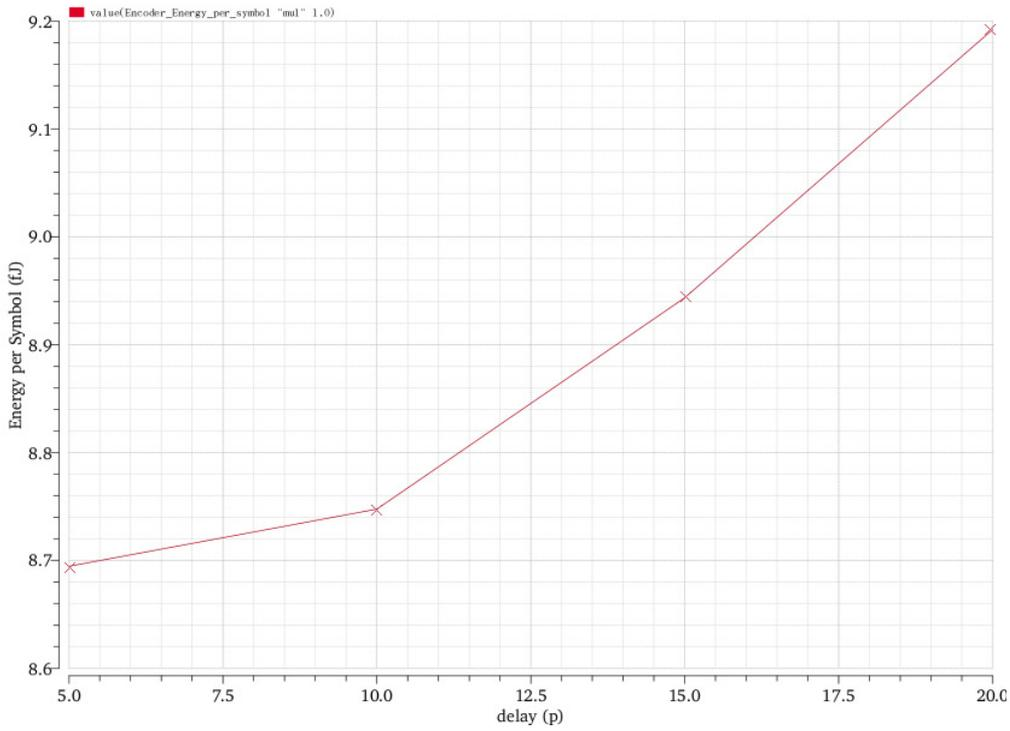
**Figure 6.14:** Energy efficiency in fJ per symbol for delay times {10 ps - 20ps} for width multiplier of 1.0.
