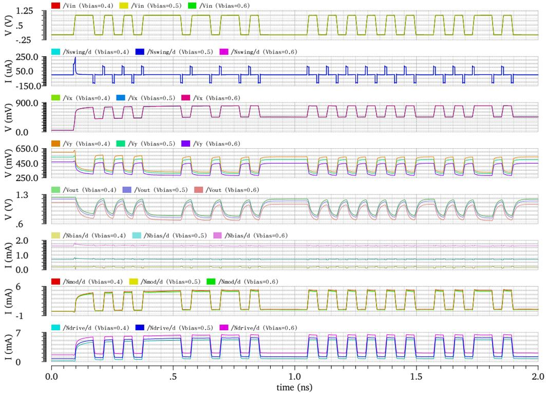
**Figure 6.16:** Transient performance of the driver slice for various values of  $V_{bias}$ . From top to bottom:  $V_{in}$ ,  $I_{swing}$ ,  $V_x$ ,  $V_y$ ,  $V_{out}$ ,  $I_{bias}$ ,  $I_{modulation}$ ,  $I_{driver}$ .
