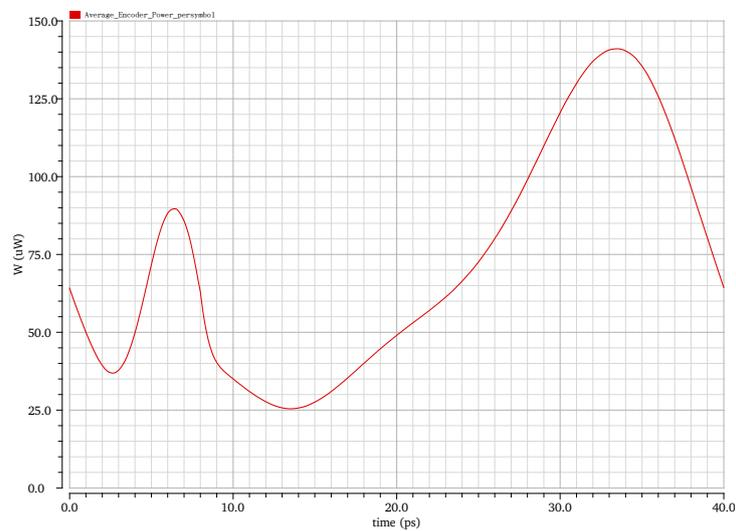
**Figure 6.8:** Average power per symbol calculated over 3 ns with random input bit streams.
