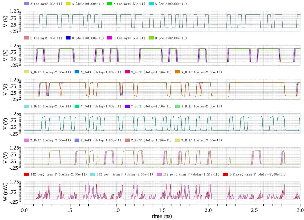
**Figure 6.13:** Transient plot of the performance of the encoder including output buffers for *width multiplier* of 1.0 and delay between the inputs of 10p - 20p. From top to bottom: the 2 input bit-streams  $A$  and  $B$ , the three outputs from the buffers  $X\_buff$ ,  $Y\_buff$  and  $Z\_buff$ , and the instantaneous Power drawn by the encoder  $I42:pwr$  including the buffers.
