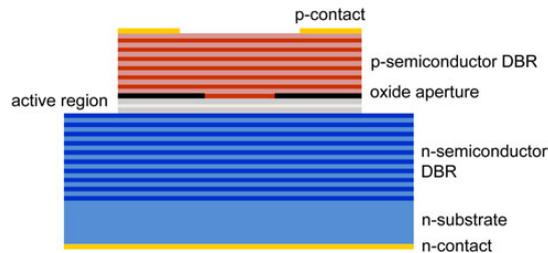
**Figure 2.2:** Cross-section of a typical VCSEL structure [27].
