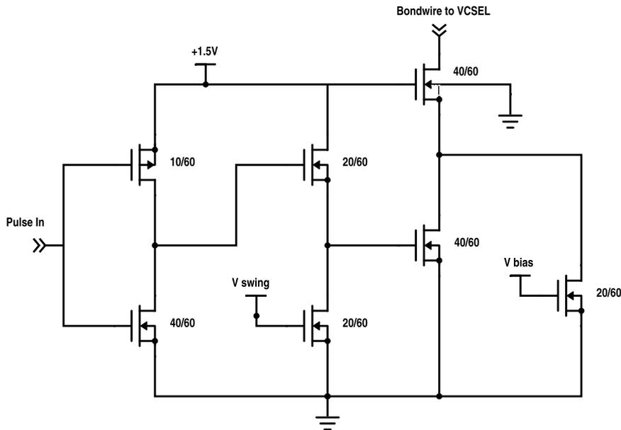
**Figure 4.4:** Schematic of a driver slice derived from [11] including a buffer inverter. The MOSFET dimensions (channel width/length) are in  $\mu\text{m}/\text{nm}$  and were used in the first test setup.
