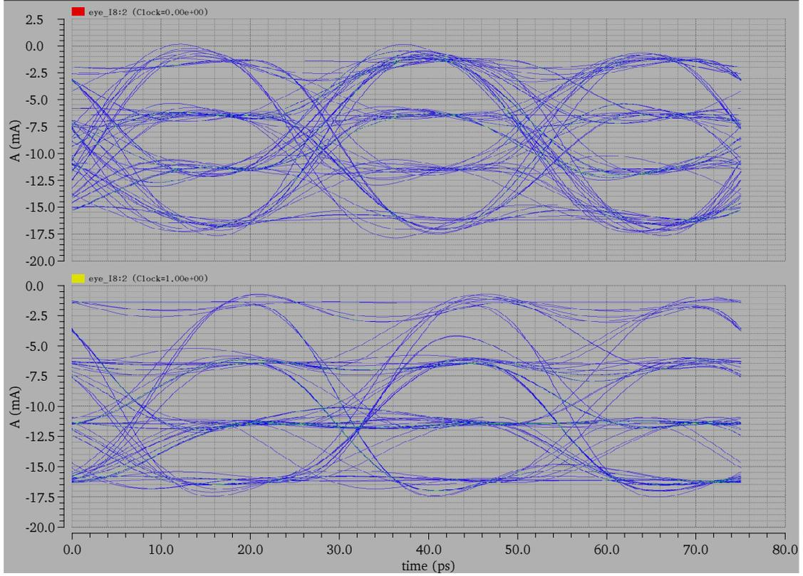
**Figure D.1:** Eye diagrams for Synchronous (top) and Asynchronous (bottom) mode operation at 40 GHz for control voltage values:  $V_b = 0.45$  V,  $V_{sw} = 0.5$  V and  $V_{body} = 3$  V, and bond wire length  $w_{bl} = 700\mu\text{m}$ .
