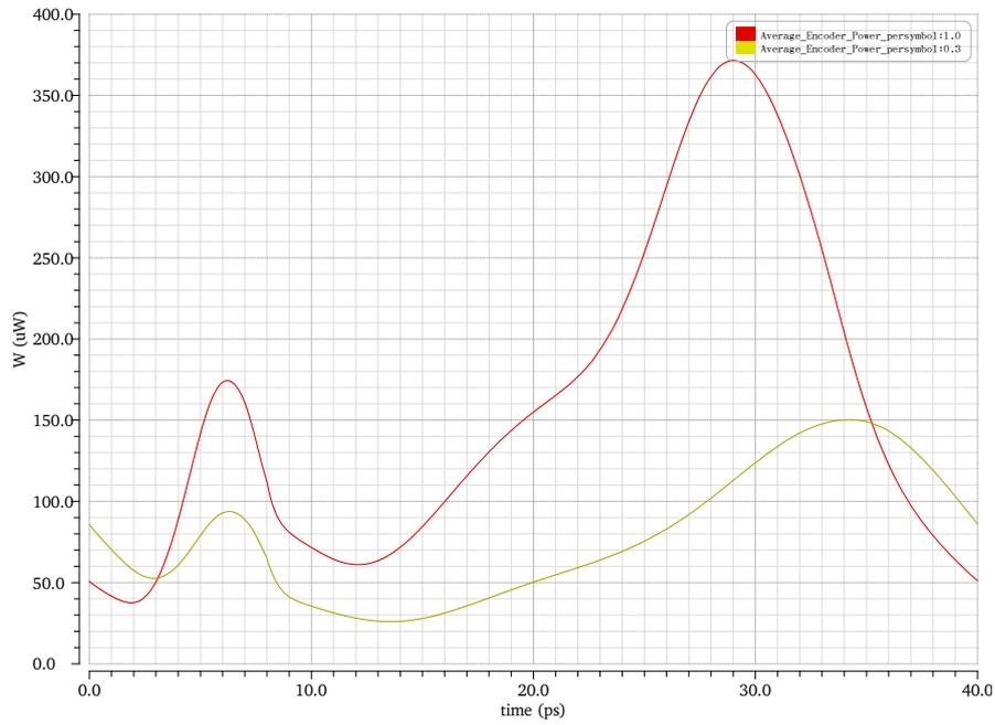
(a) [Instantaneous power of a single symbol averaged.] (40 ps) averaged over the total simulation time.
