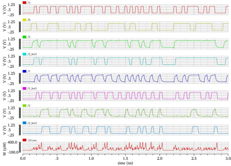
**Figure 6.5:** Transient plot of the performance of the encoder without including output buffers for *width multiplier* of 0.3. From top to bottom: the 2 input bit-streams  $A$  and  $B$ , the three outputs of the encoder  $X$ ,  $Y$  and  $Z$  along with the respective outputs from the buffers  $X\_buff$ ,  $Y\_buff$  and  $Z\_buff$ , and the instantaneous Power drawn by the encoder  $I42:pwr$  including the buffers.
