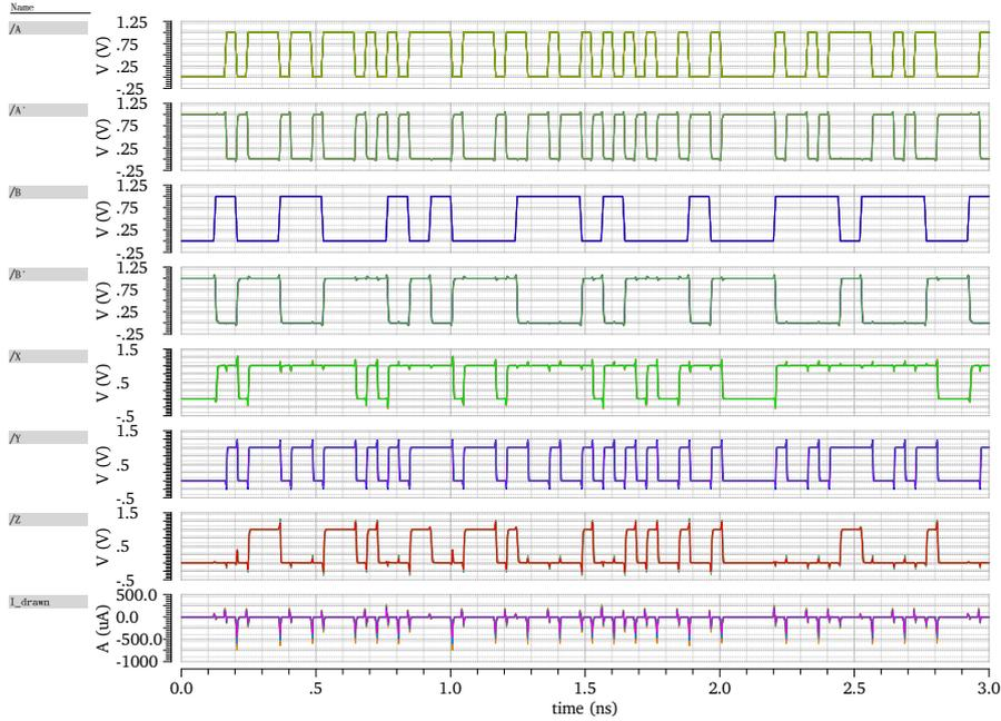
**Figure 6.4:** Transient plot of the performance of the encoder without latches and output buffers for values of *width multiplier* between 0.3, 1. From top to bottom: the 2 input bit-streams  $A$  and  $B$  and their inverted counterparts  $A'$  and  $B'$ , the three outputs of the encoder  $X$ ,  $Y$  and  $Z$ , and the total instantaneous current drawn by the encoder.
