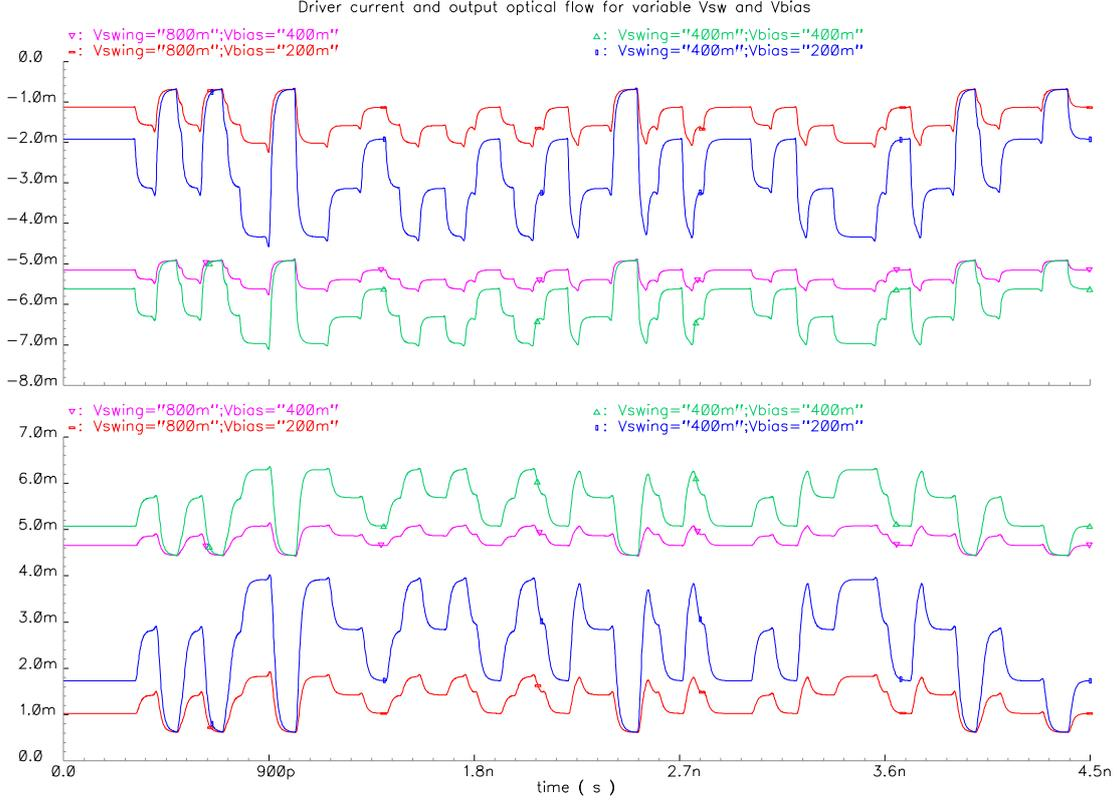
**Figure 5.3:** Simulation of the 65 nm drive for  $V_{bias} = \{200, 400\} \text{ mV}$  and  $V_{swing} = \{400, 800\} \text{ mV}$ . Top: The current at the output of the driver - cathode of the VCSEL. Bottom: the optical current at the output of the VCSEL.
