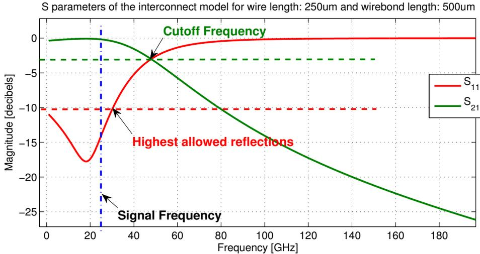
**Figure 5.4:** Graph of the S-parameters of the driver load including interconnects for wire length  $w_l = 250 \mu m$  and bond wire length  $w_b = 500 \mu m$ .
