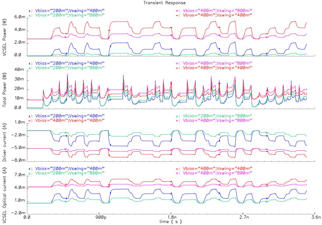
**Figure 5.6:** Power consumption of the 65 nm driver circuit vs the laser current and optical current. The parametric analysis is for  $V_{bias} = \{200, 400\} mV$  and  $V_{swing} = \{400, 800\} mV$ .
