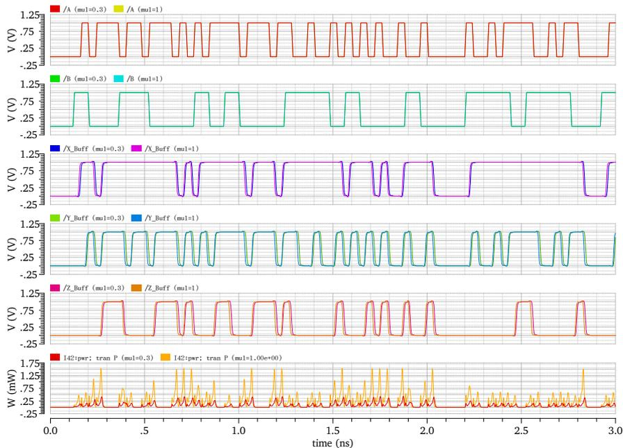
**Figure 6.9:** Transient plot of the performance of the encoder, including output buffers, for values of *width multiplier* between 0.3, 1. From top to bottom: the 2 input bit-streams *A* and *B*, the three outputs of the encoder *X\_buff*, *Y\_buff* and *Z\_buff*, and the instantaneous power of the encoder including the output buffers.
