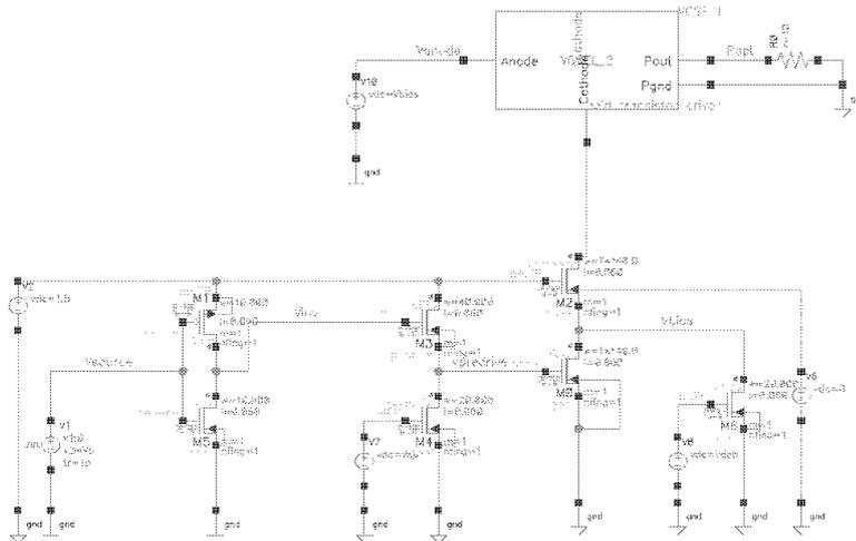
**Figure B.1:** Cadence circuit model of the 65 nm driver and the VCSEL load.
