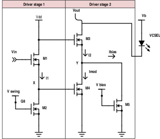
**Figure 4.5:** Circuit schematic of a single driver slice divided into its two stages. The source follower stage (stage 1) and the Cascode stage (stage 2).
