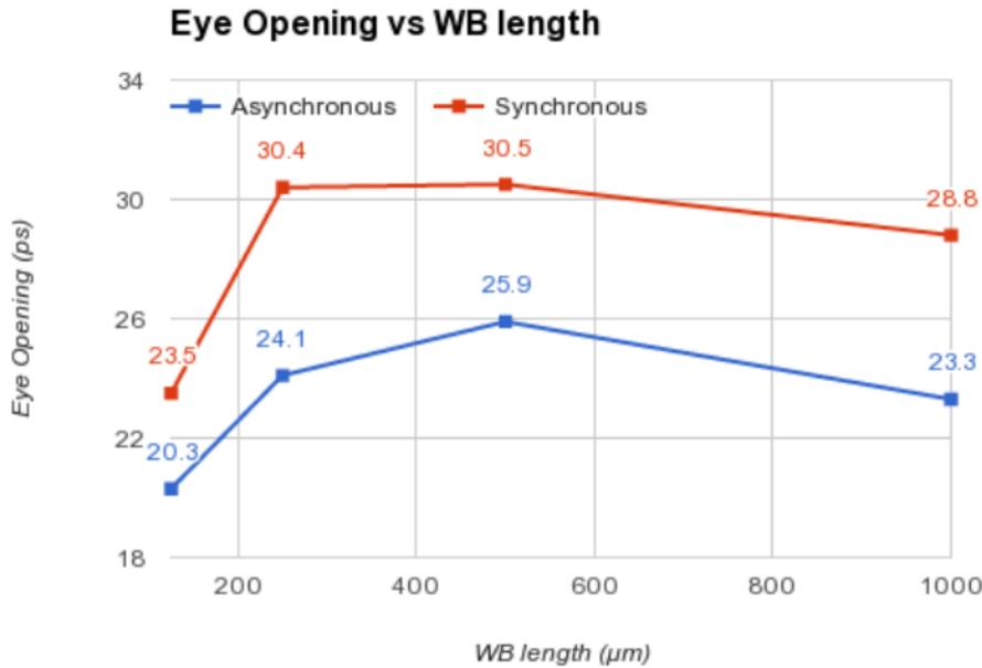
**Figure 7.5:** Eye opening vs wire-bond inductance for synchronous and asynchronous mode.
