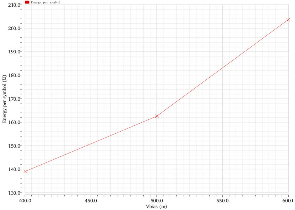
**Figure 6.17:** Energy efficiency in fJ per symbol of a driver slice for values of  $V_{bias}=\{0.4, 0.5, 0.6\}$ .
