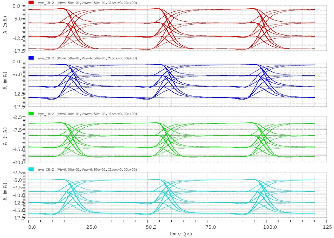
**Figure 7.3:** Eye diagrams in Synchronous mode for the extreme corners for the control voltages  $V_{bias}$ ,  $V_{sw}$  and  $V_{body} = 3$  V. The graphs are from top to bottom: Red:  $V_{bias} = 450$  mV,  $V_{sw} = 450$  mV, Blue:  $V_{bias} = 450$  mV,  $V_{sw} = 650$  mV, Green:  $V_{bias} = 600$  mV,  $V_{sw} = 450$  mV, Cyan:  $V_{bias} = 600$  mV,  $V_{sw} = 650$  mV
