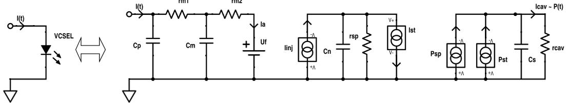
(b) The electrical equivalent circuit of the VCSEL chip.
