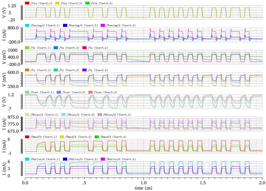
**Figure 6.18:** Transient performance of the driver slice for various values of  $V_{sw}$ . From top to bottom:  $V_{in}$ ,  $I_{swing}$ ,  $V_x$ ,  $V_y$ ,  $V_{out}$ ,  $I_{bias}$ ,  $I_{modulation}$ ,  $I_{driver}$ .
