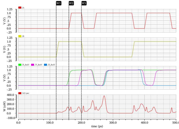
**Figure 6.7:** Transient plot of the averaging window to calculate the average power per symbol. From top to bottom: the 2 input bit-streams  $A$  and  $B$ , the three outputs from the buffers  $X\_buff$ ,  $Y\_buff$  and  $Z\_buff$ , and the instantaneous power drawn by the encoder  $I42:pw$  including the buffers. The three markers represent the the borders between two consecutive windows or symbols.
