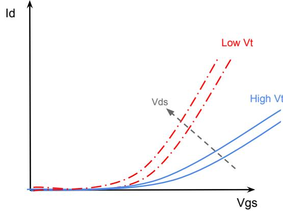
**Figure 6.2:** Graphic representation of the  $I-V_{gs}$  characteristic for low and high threshold N-MOS devices.
