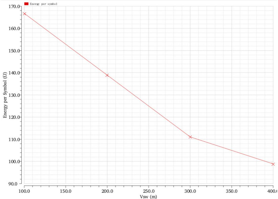
**Figure 6.19:** Energy efficiency in fJ per symbol for different values of  $V_{sw}$ .
