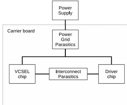
Figure 4.1: Block diagram of the system.
