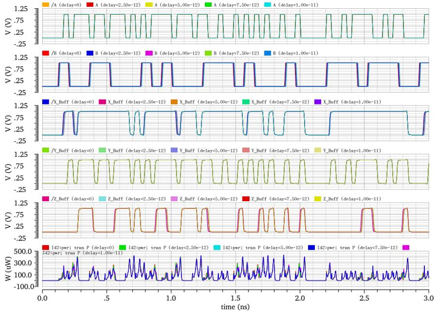
**Figure 6.11:** Transient plot of the performance of the encoder including output buffers for *width multiplier* of 0.3 and delay between the inputs of 0p - 11p. From top to bottom: the 2 input bit-streams  $A$  and  $B$ , the three outputs of the encoder  $X$ ,  $Y$  and  $Z$  along with the respective outputs from the buffers  $X\_buff$ ,  $Y\_buff$  and  $Z\_buff$ , and the instantaneous power drawn by the encoder  $I42:pwr$  including the buffers.
