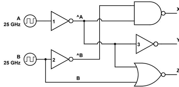
**Figure 4.3:** Logic diagram of the binary-to-thermometer Gray encoder.
