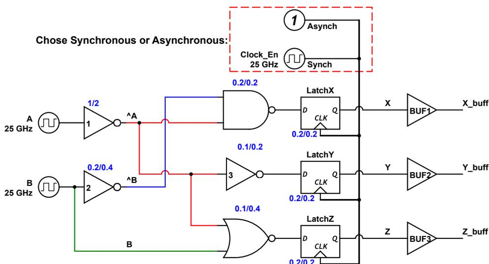
**Figure 6.3:** Schematic of the binary to thermometer Gray encoder including transistor relative sizes (N-mos/P-mos) and output driving buffers. The widths are in relation to a unit inverter defined in order to protect the sensitive process parameters covered by the NDA.
