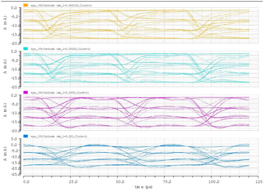
**Figure 7.6:** Eye diagrams in Asynchronous mode for various lengths of the wire-bonds.
