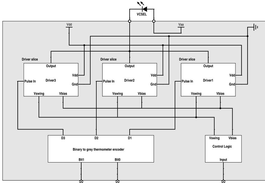
Figure 4.2: Block schematic of the complete driver architecture.
