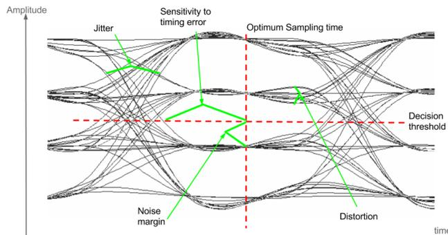
**Figure 3.3:** Sample eye diagram along with some of the signal figures that can be extracted by it.
