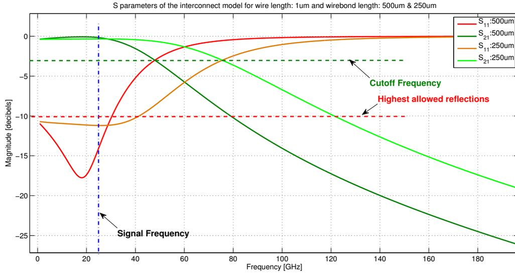
**Figure D.2:** Graph of the S-parameters of the driver load including interconnects for wire length  $w_l = 1 \mu m$  and bond wire length  $w_{bl} = \{250, 500\} \mu m$ .
