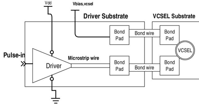
**Figure 2.5:** Proposed integration topology of the driver-VCSEL system with wire-bonding including the parasitics.
