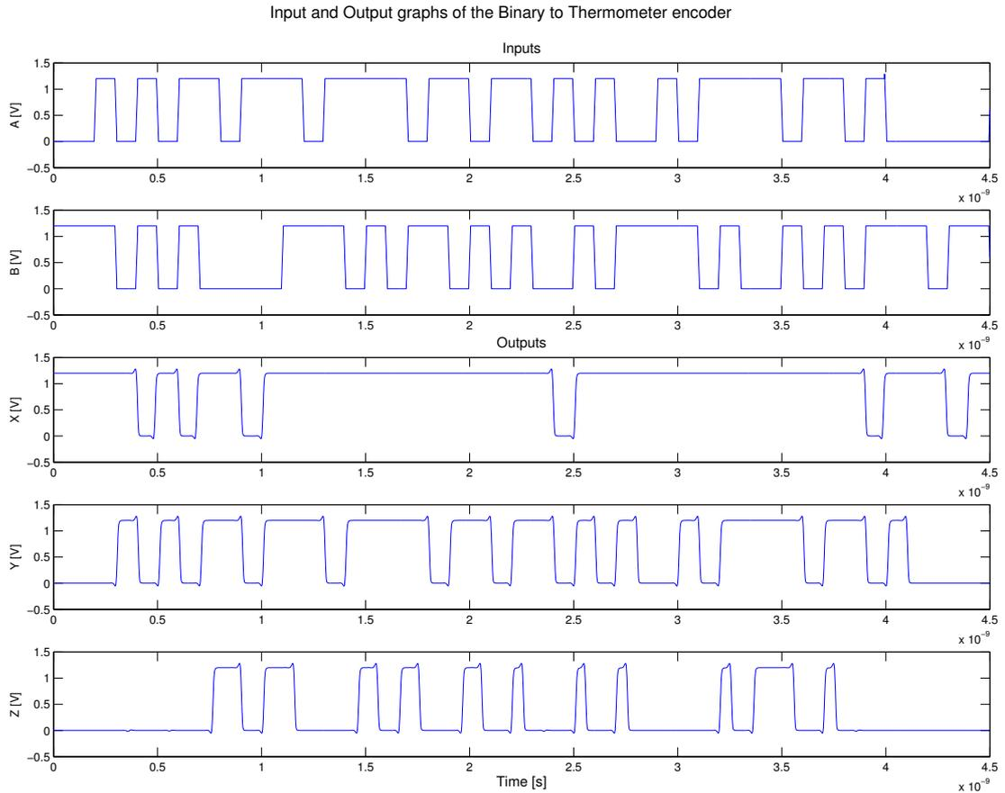
**Figure 5.1:** Simulation of the binary to thermometer encoder. From top to bottom:  $A$  and  $B$  are the input bit streams at 10 GHz,  $X$ ,  $Y$  and  $Z$  are the outputs of the Thermometer encoder.
