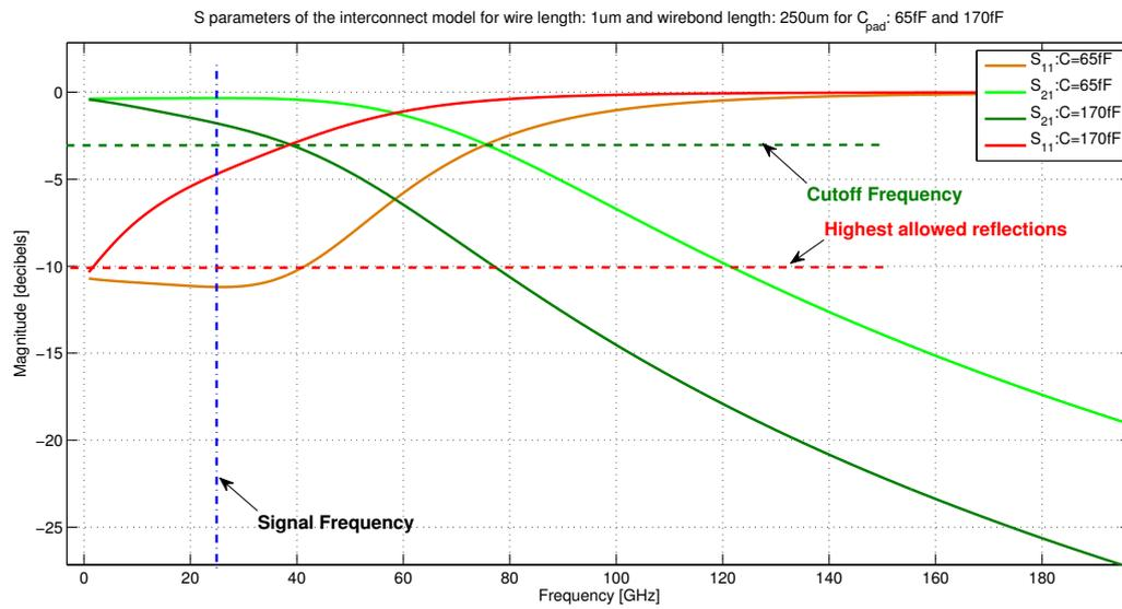
**Figure D.4:** Graph of the S-parameters of the driver load including interconnects for wire length  $w_l = 1 \mu\text{m}$  and bond wire length  $wb_l = 250 \mu\text{m}$  and variable bond-pad capacitance values.
