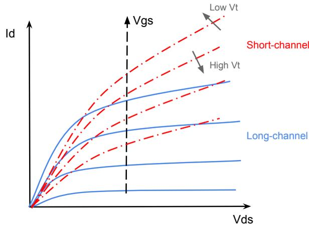
**Figure 6.1:** Graphic representation of the  $I$ - $V_{ds}$  characteristic for short and long channel N-MOS devices for various values of  $V_{GS}$ .
