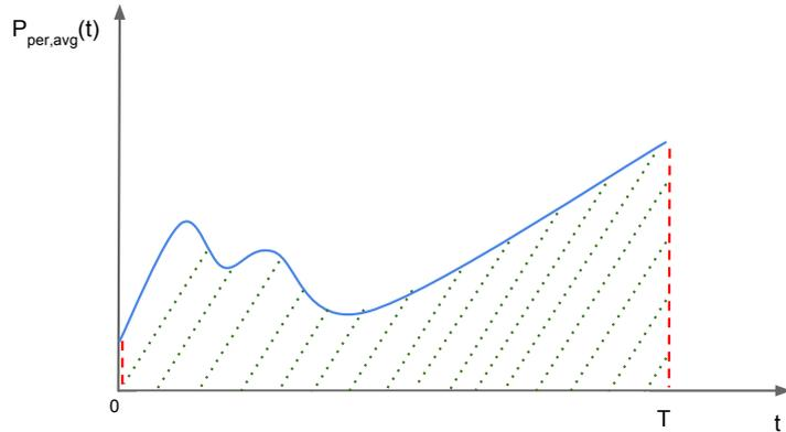
**Figure 3.2:** Averaged instantaneous power of a symbol. The dotted lines represent the surface given by the integral that represents the energy per symbol.
