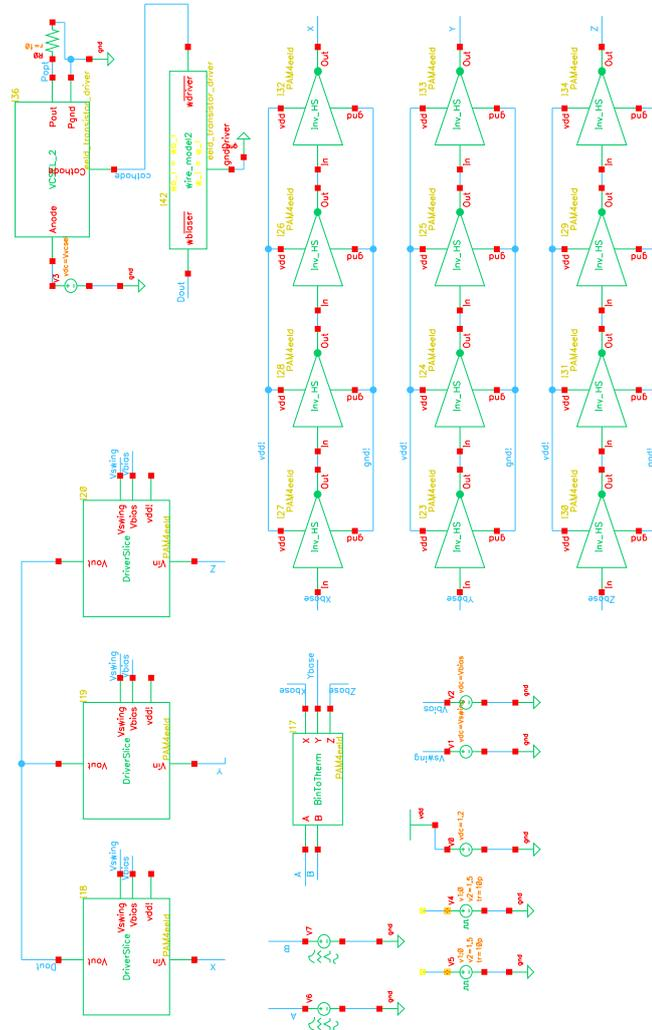
**Figure B.2:** Schematic printout of the Test Bench used for characterizing the 65nm Driver design.
