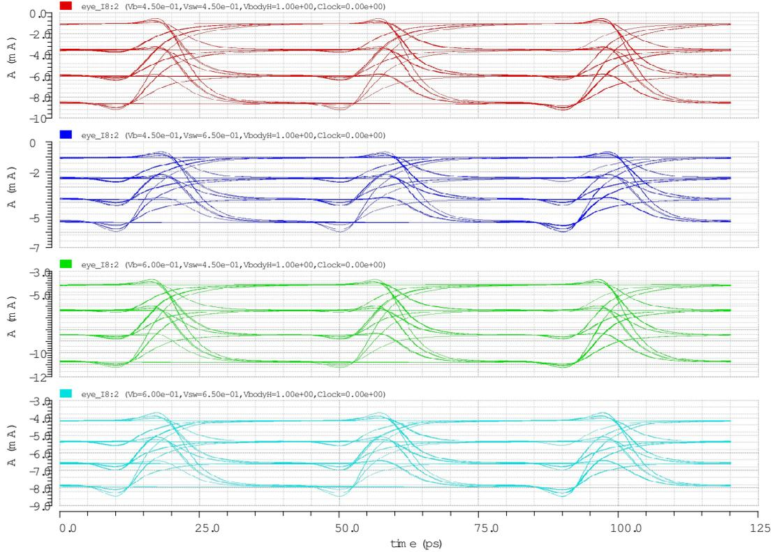
**Figure 7.4:** Eye diagrams in Synchronous mode for the extreme corners for the control voltages  $V_{bias}$ ,  $V_{sw}$  and  $V_{body} = 1$  V. The graphs are from top to bottom: Red:  $V_{bias} = 450$  mV,  $V_{sw} = 450$  mV, Blue:  $V_{bias} = 450$  mV,  $V_{sw} = 650$  mV, Green:  $V_{bias} = 600$  mV,  $V_{sw} = 450$  mV, Cyan:  $V_{bias} = 600$  mV,  $V_{sw} = 650$  mV
