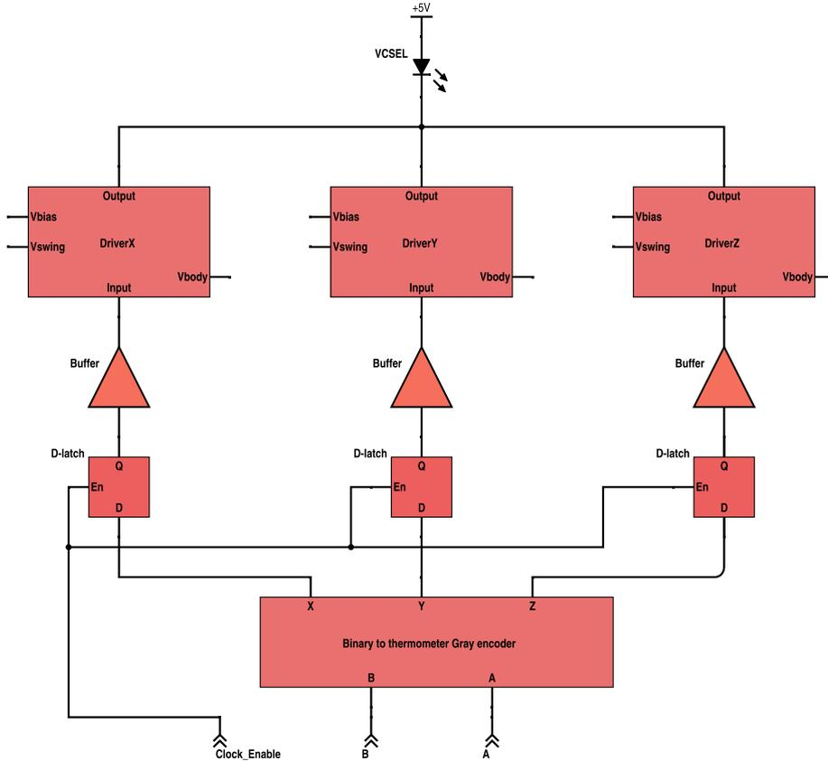
**Figure 7.1:** Block diagram of the final driver layout. The  $V_{dd}$  and  $Gnd$  on each block are implied and were left out of the schematic for clarity reasons.
