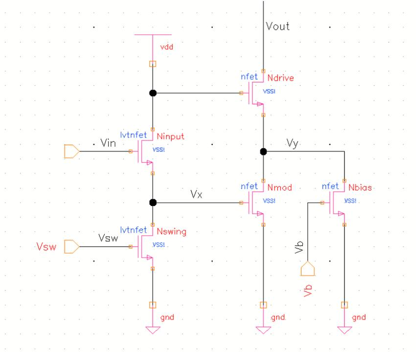
**Figure 6.15:** Schematic of the test implementation of the driver slice on Cadence ADS.
