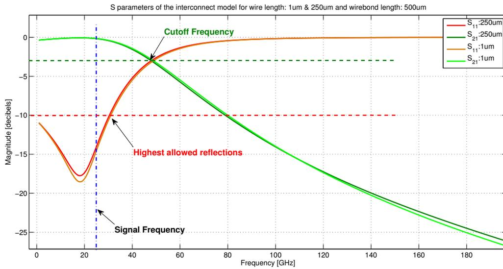
**Figure D.3:** Graph of the S-parameters of the driver load including interconnects for wire length  $w_l = \{1, 250\} \mu m$  and bond wire length  $w_{bl} = 250 \mu m$ .
