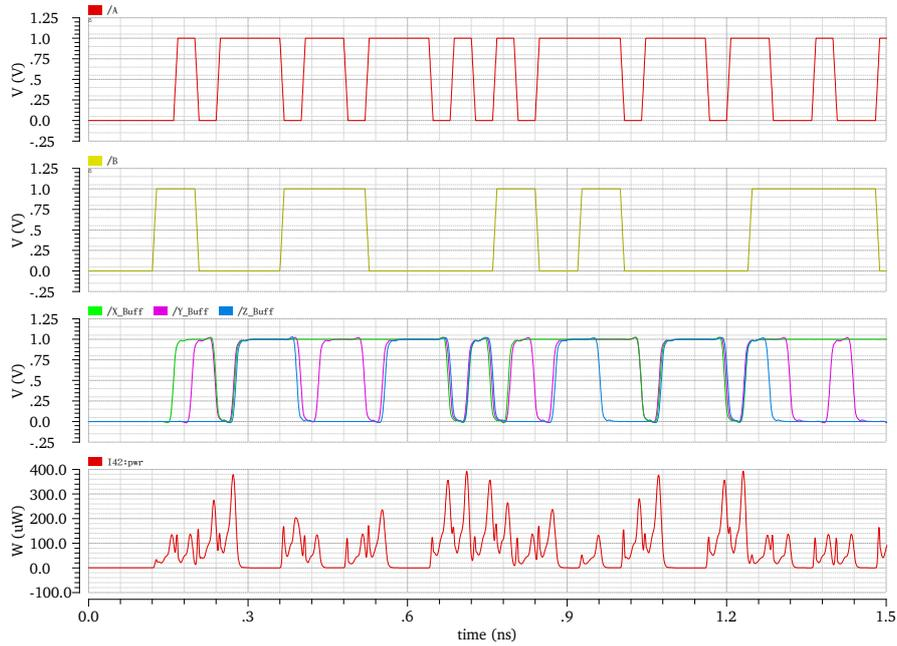
**Figure 6.6:** Transient plot of the performance of the encoder without including output buffers for *width multiplier* of 0.3. From top to bottom: the 2 input bit-streams *A* and *B*, the three outputs from the buffers *X\_buff*, *Y\_buff* and *Z\_buff*, and the instantaneous Power drawn by the encoder *I42:pw* including the buffers.
