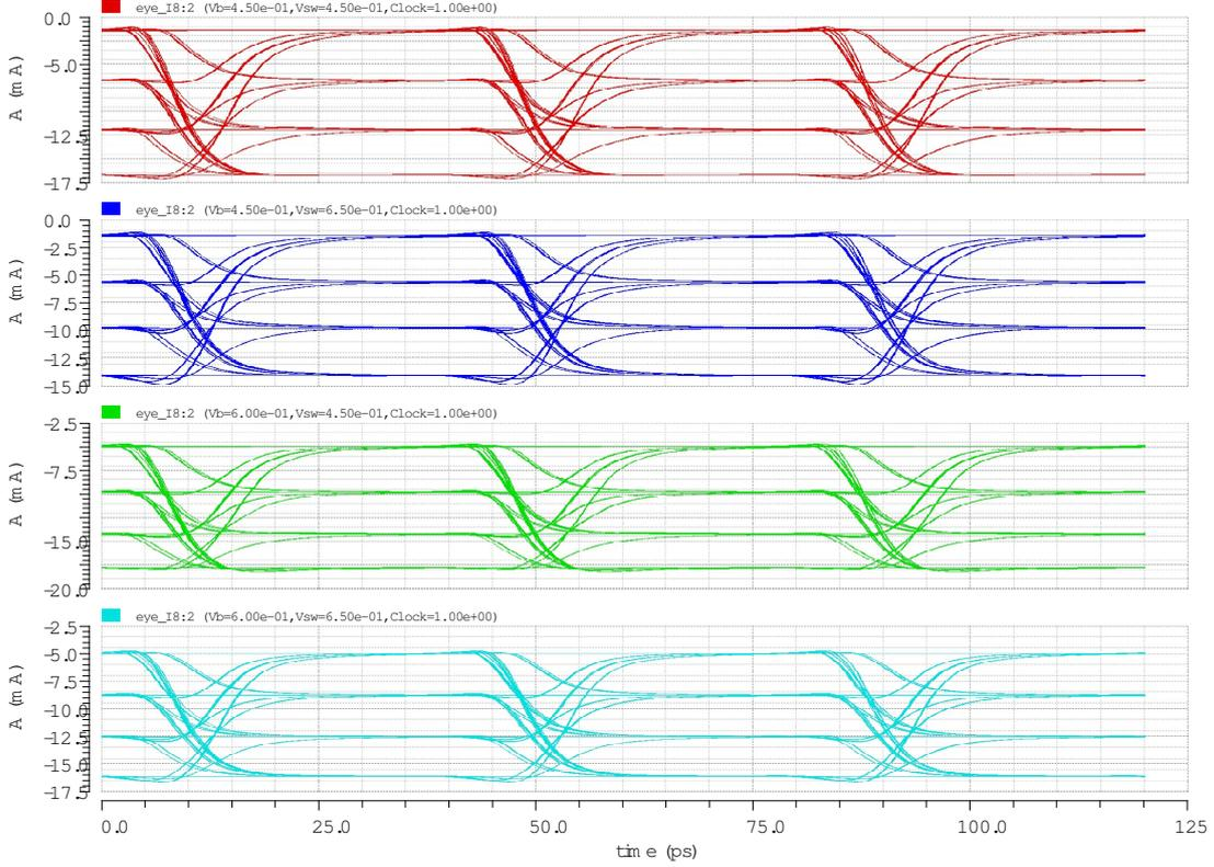
**Figure 7.2:** Eye diagrams in Asynchronous mode for the extreme corners for the control voltages  $V_{bias}$ ,  $V_{sw}$  and  $V_{body} = 3$  V. The graphs are from top to bottom: Red:  $V_{bias} = 450$  mV,  $V_{sw} = 450$  mV, Blue:  $V_{bias} = 450$  mV,  $V_{sw} = 650$  mV, Green:  $V_{bias} = 600$  mV,  $V_{sw} = 450$  mV, Cyan:  $V_{bias} = 600$  mV,  $V_{sw} = 650$  mV
