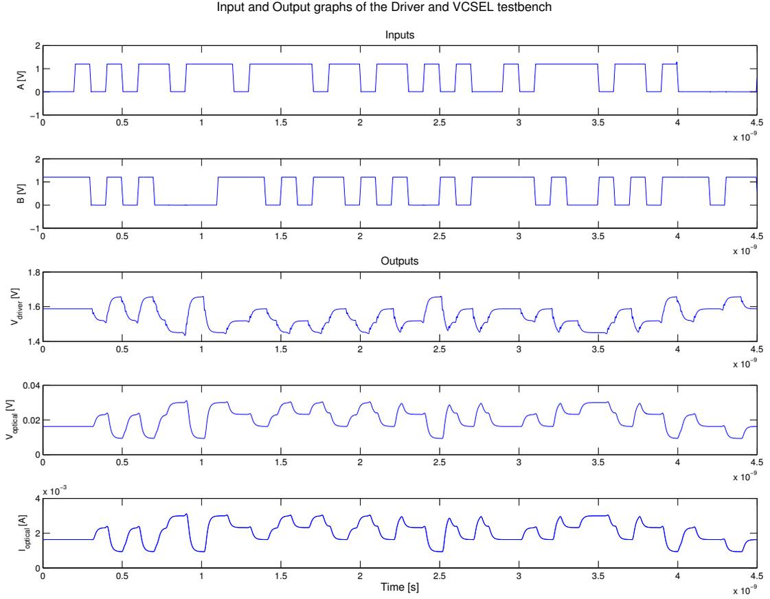
**Figure 5.2:** Simulation of the complete drive. From top to bottom:  $A$  and  $B$  are the input bit streams at 10 GHz,  $V_{driver}$  is the output voltage of the driver, and  $V_{driver}$ ,  $I_{optical}$  are the outputs of the VCSEL model.
