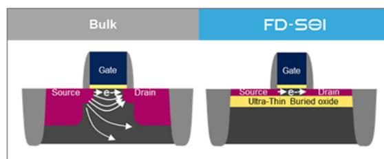
**Figure 2.4:** Structural differences between bulk and FDSOI 28 nm technologies [39].
