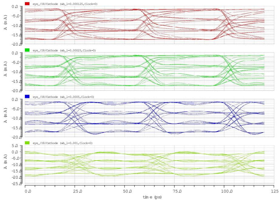
**Figure 7.7:** Eye diagrams in Synchronous mode for various lengths of the wire-bonds.
