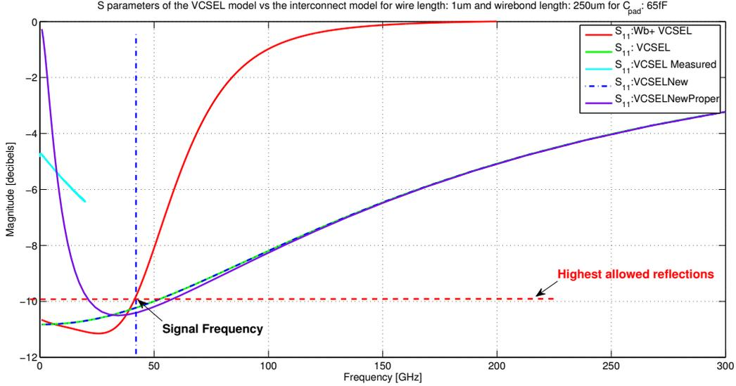
**Figure 5.5:** Graph of the S-11 parameters of the VCSEL load. *Red:* S-11 of the VCSEL including the wirebonds. *Green:* S-11 of the VCSEL model described in Verilog. *Cyan:* Measured S-11 from the fabricated VCSEL die. *Blue dashed:* Verilog-free VCSEL electrical equivalent model. *Purple:* VCSEL model with dynamic resistance modeling.
