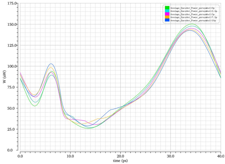
(a) Instantaneous power of a single symbol (40 ps) averaged over the total simulation time .
