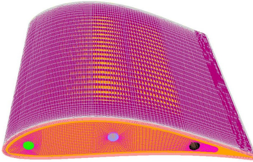
Figure 7.4: Vane Mesh. The three cylinders inside are the three heaters
