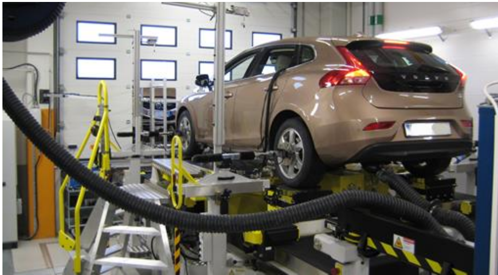
Figure 5 - Vehicle installed in the SPMM 5000 K&C measurement machine.
