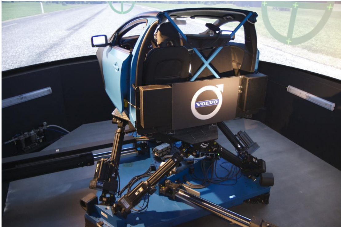
Figure 2 - The moving base driving simulator used at Volvo Cars.
