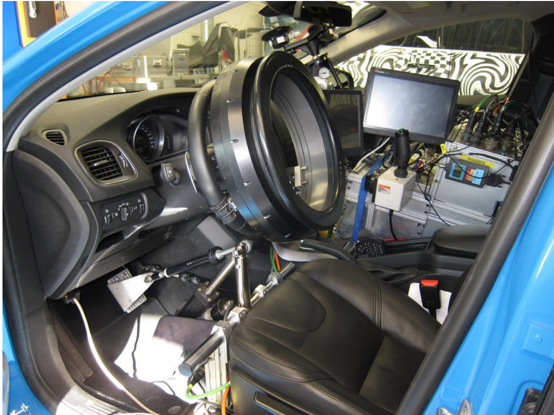
Figure 11 - Driving robots used during physical testing.
