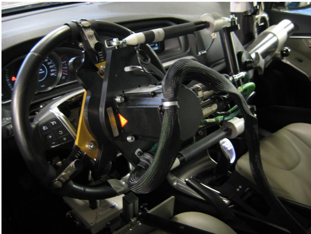
Figure 6 - Steering robot used during K&C measurements.
