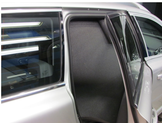
Figure 47: A heavy layer on side window.
