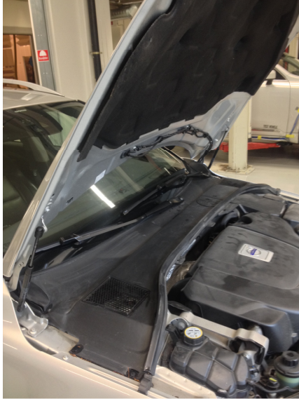
Figure 38: Cowl cavity shape for real car.
