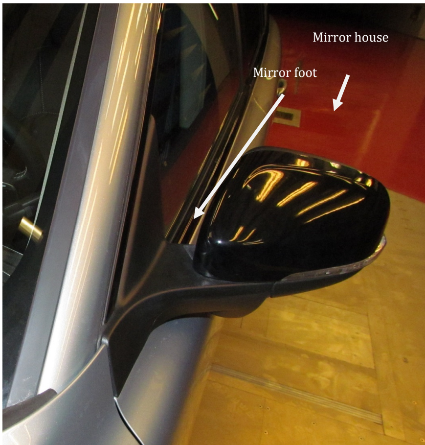
Figure 7: Locations for exterior measurement.
