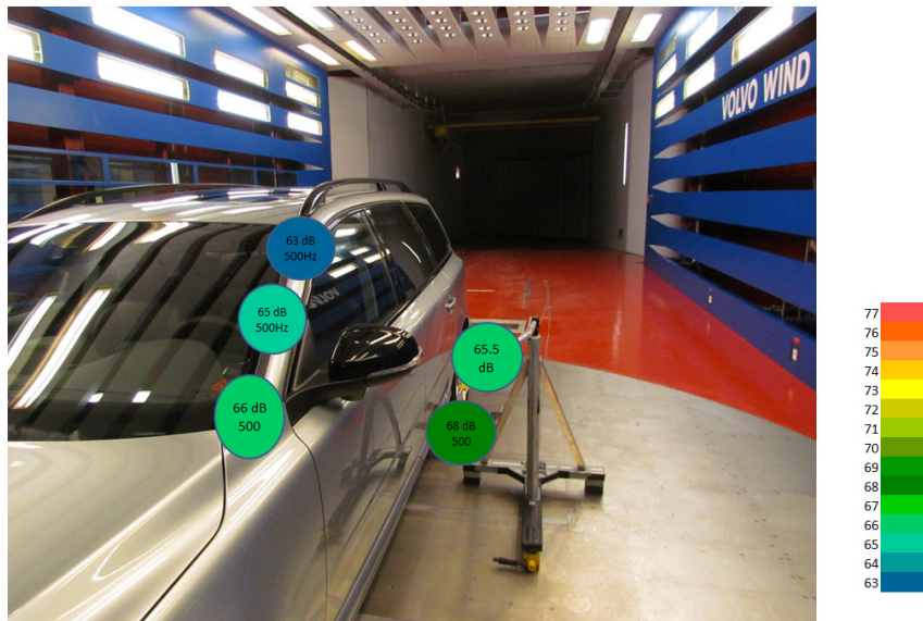
Figure 8: Maximum intensity at each measurement location at wind speed 90 km/h.
