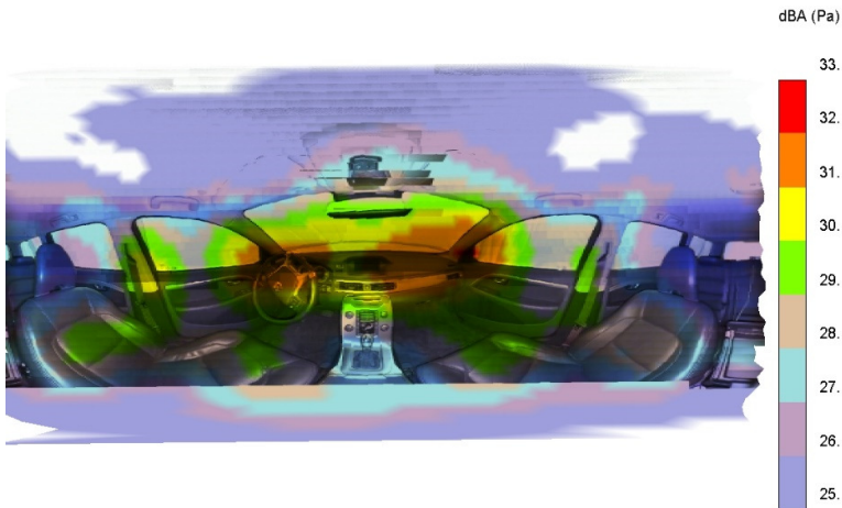
Figure 60: Interior noise radiation pattern for conf. 3 at [0s 15s], [1790Hz 2240 Hz] at wind speed 130 Km/h.
