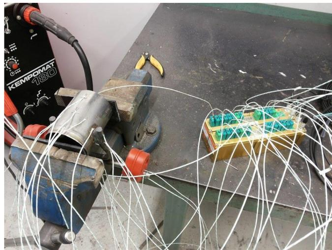
**Figure 3.2 Experimental Setup and Placement of Thermocouples**
