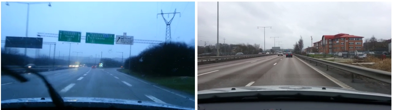
Figure 2.3: Example images depicting how hard it might be to determine distances in a frame from the video captured. In the right image, the black car (in the same lane) and the white car (in the left lane) are almost next to each other but in reality the white car already passed the black. But how far ahead of the black is the white?
