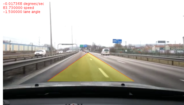
Figure 4.12: A frame where the lane markers have drifted to the right as the car is moving from the left to the right lane. The drift occurs because no new lines are detected and therefore the old ones are kept.
