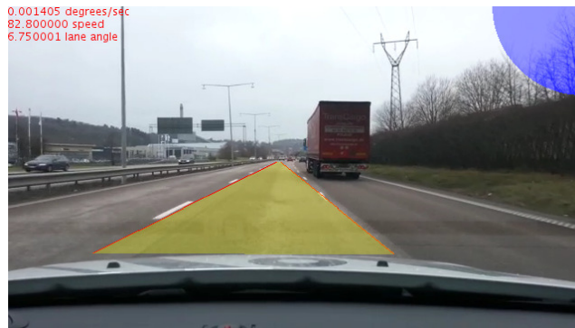
Figure 3.8: An example depicting the activated LDW, here crossing the lane to the right. The blue circle in the top right corner is the LDW indicating a right turn.
