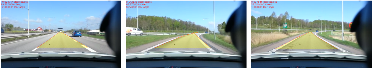
(a) When driving on a straight road the far field is just the extension of the straight lines from near field detection, which is fairly robust. (b) The right line does not trace the curve of the line, but the safety zone is decent anyway. (c) A curve farther ahead in the driving lane is not detected by the algorithm since the GPS has not reacted yet.
