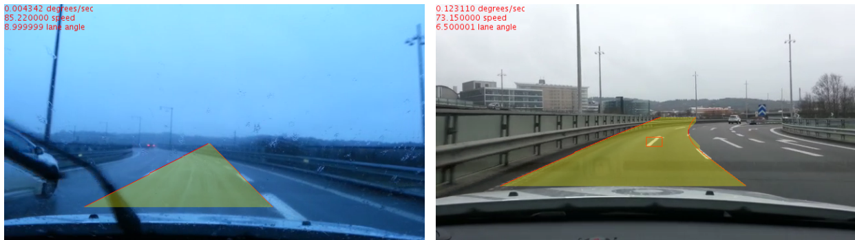
(a) Example frame where the road is turning but the GPS bearing derivative is claiming something else. Notice that the value described as degrees/sec is relatively small and positive (0.004), which indicates a slight turn to the right. (b) Example frame where the detected lane is decent, but the crash barrier is impacting the results slightly.
