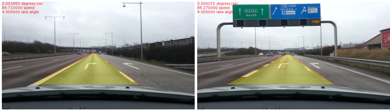
Figure 4.10: Examples of arrows on the lane that are not detected and detected respectively.
