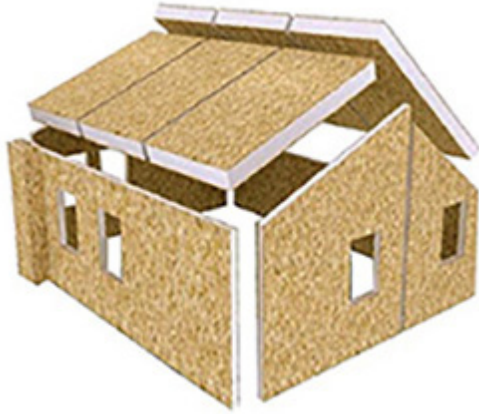
figure 44. SIP panels principle
