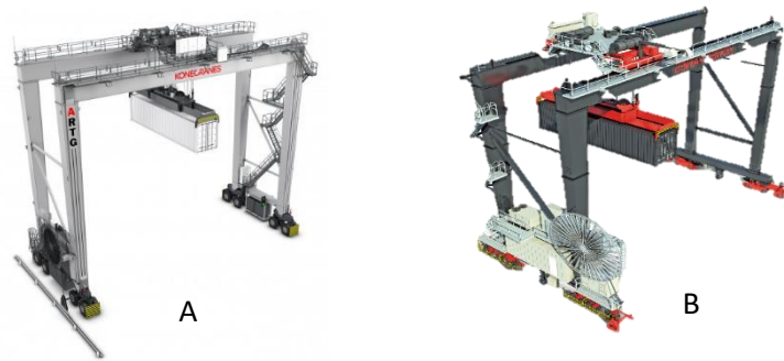
Figure 20: Yard cranes: A) RTGC, B) RGC
