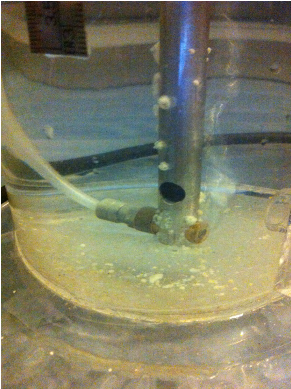
Figure 4.2: Air bubbles released from the air hose at the bottom of the tube during a measurement. 23
