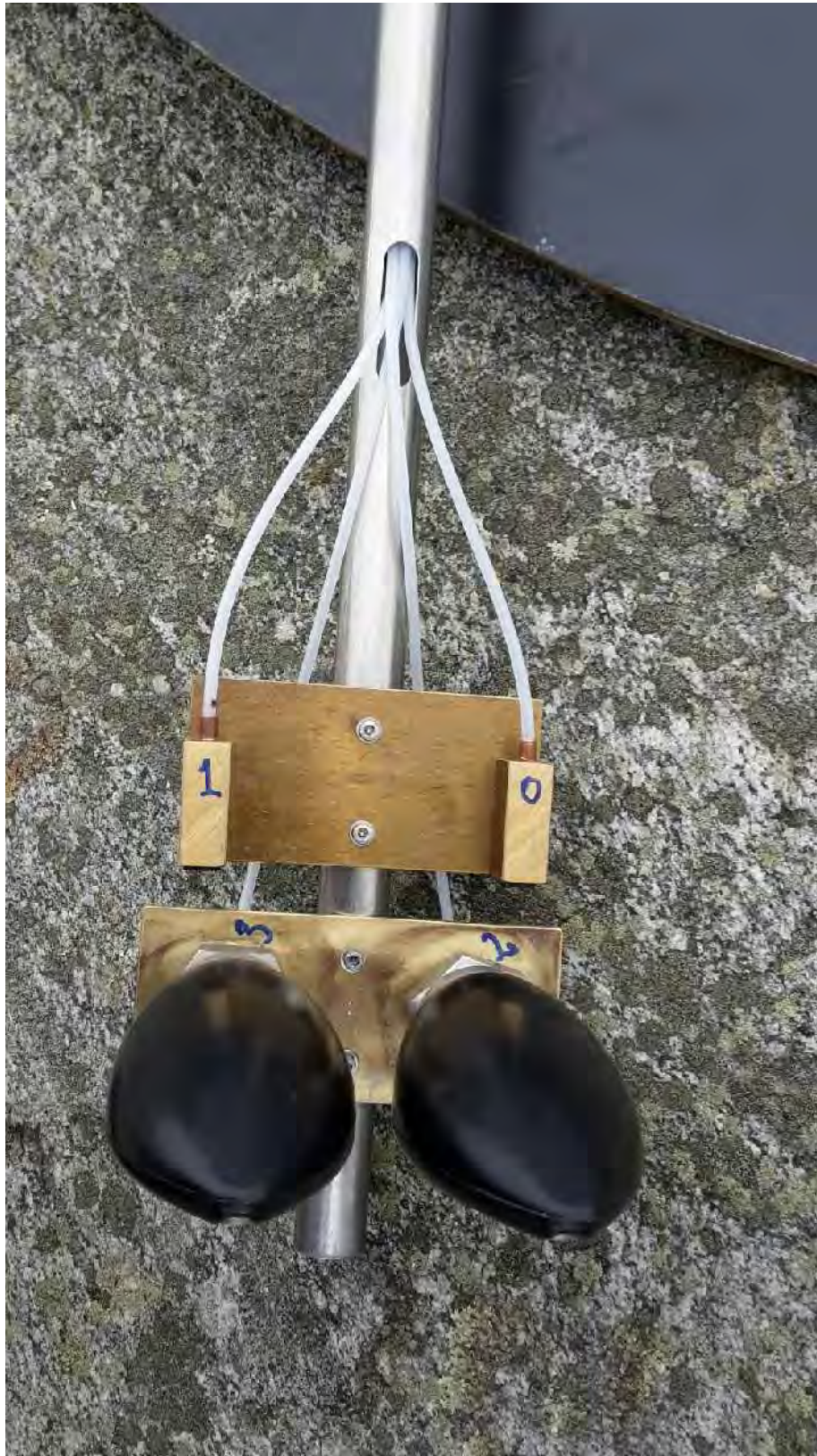
Figure 5.7: The two types of nozzles fastened to a steel rod just before they were installed in the well.
