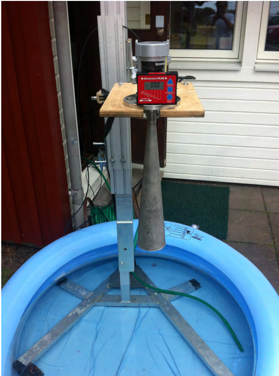
Figure 4.19: The radar placed above the pool with the inclinometer placed on top. The unit is mounted on a plate which is moveable in all directions.
