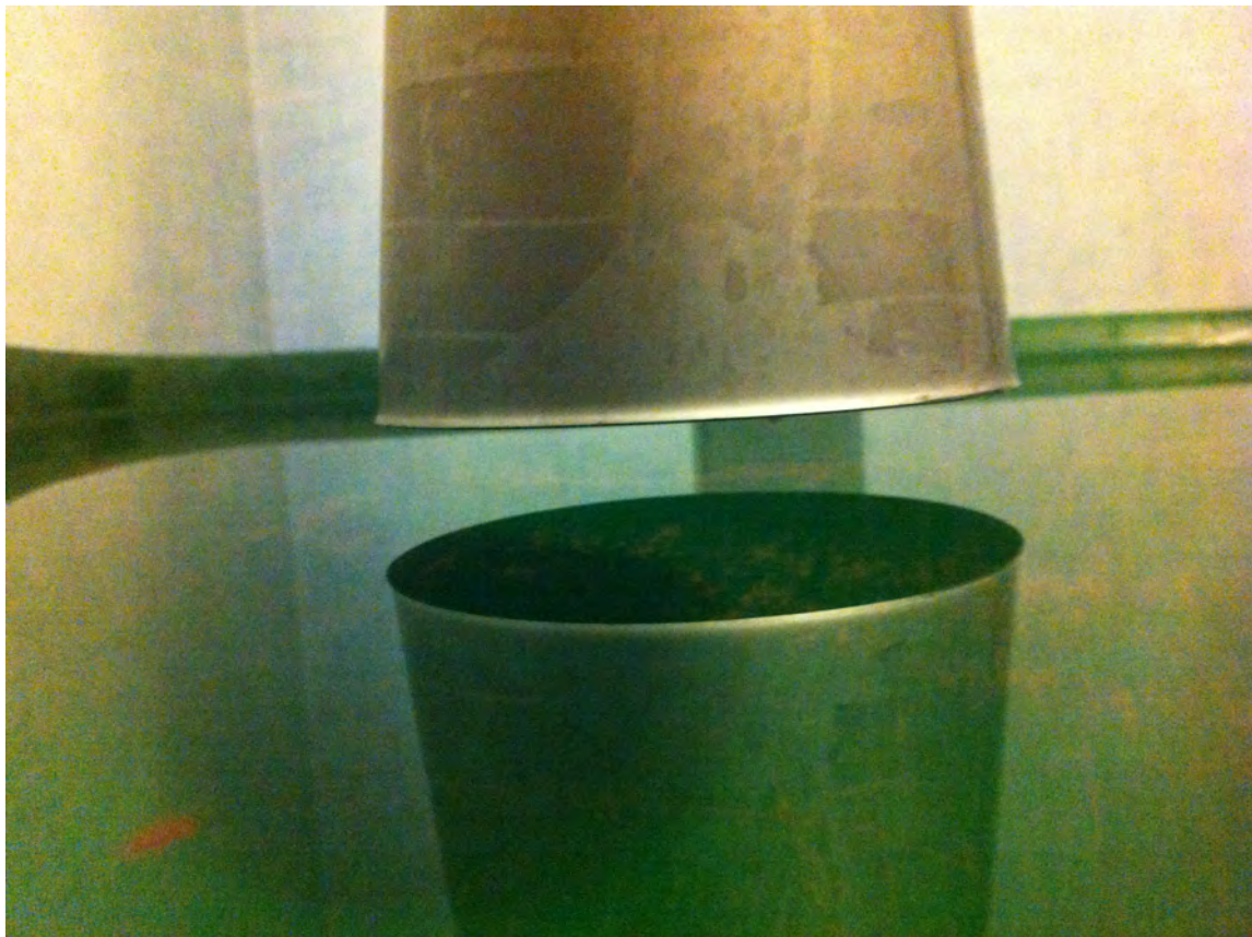
Figure 4.14: The radar horn placed just over the water surface ( d = 5 mm).
