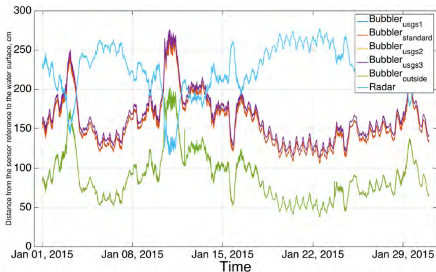
Figure 5.9: The raw data from the 4 bubble sensors in the well and the bubble sensor outside the well together with the radar. Since the radar measure the distance from above down to the water surface the data is inverted in respect to the bubbles sensor data. The bubble sensors in the well are paired into two groups were one group is fitted with the new nozzle and placed at height hrad + h_1 and the other with the original nozzle and placed at height hrad + h_2 .
