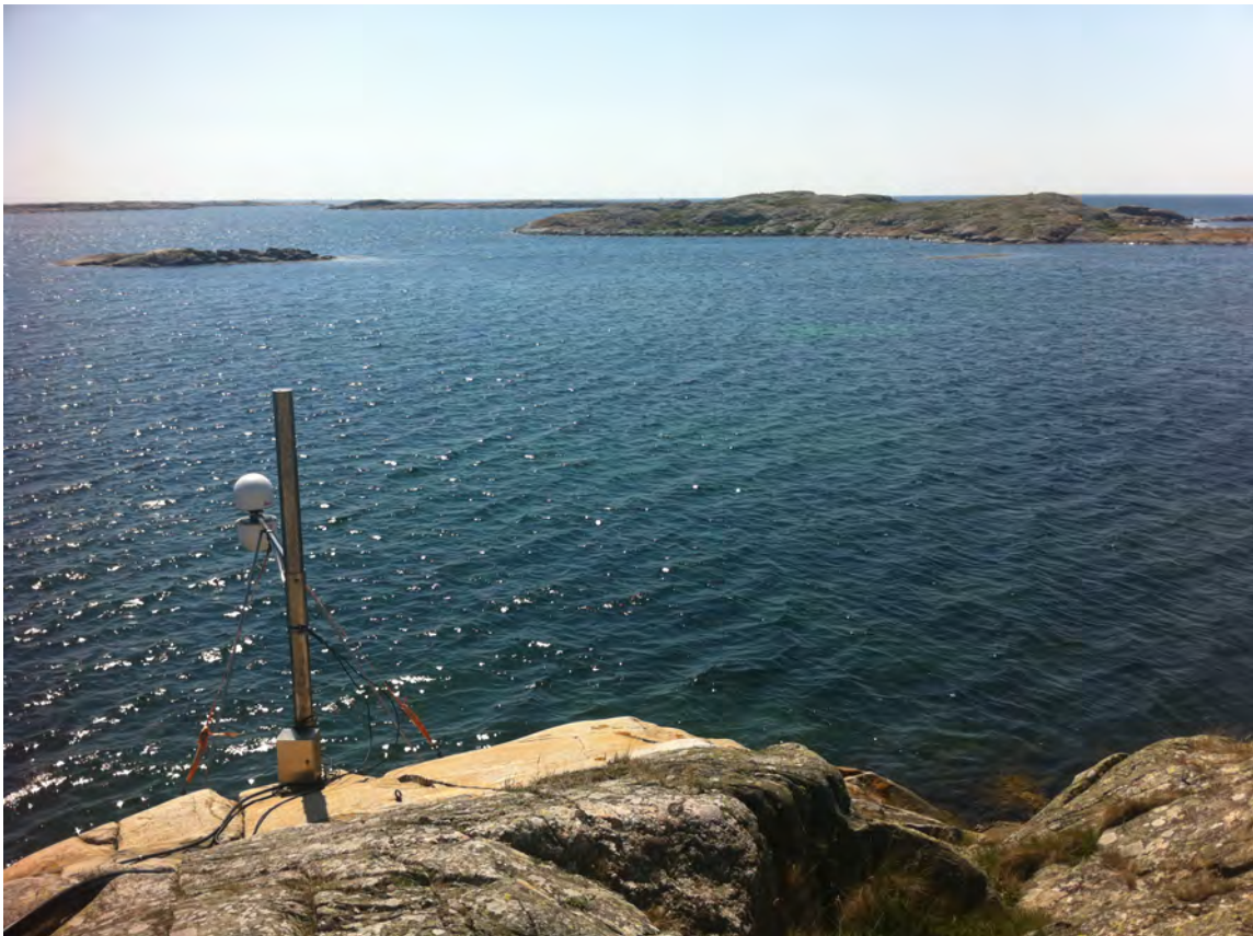
Figure 1.3: The GNSS mareograph at Onsala
