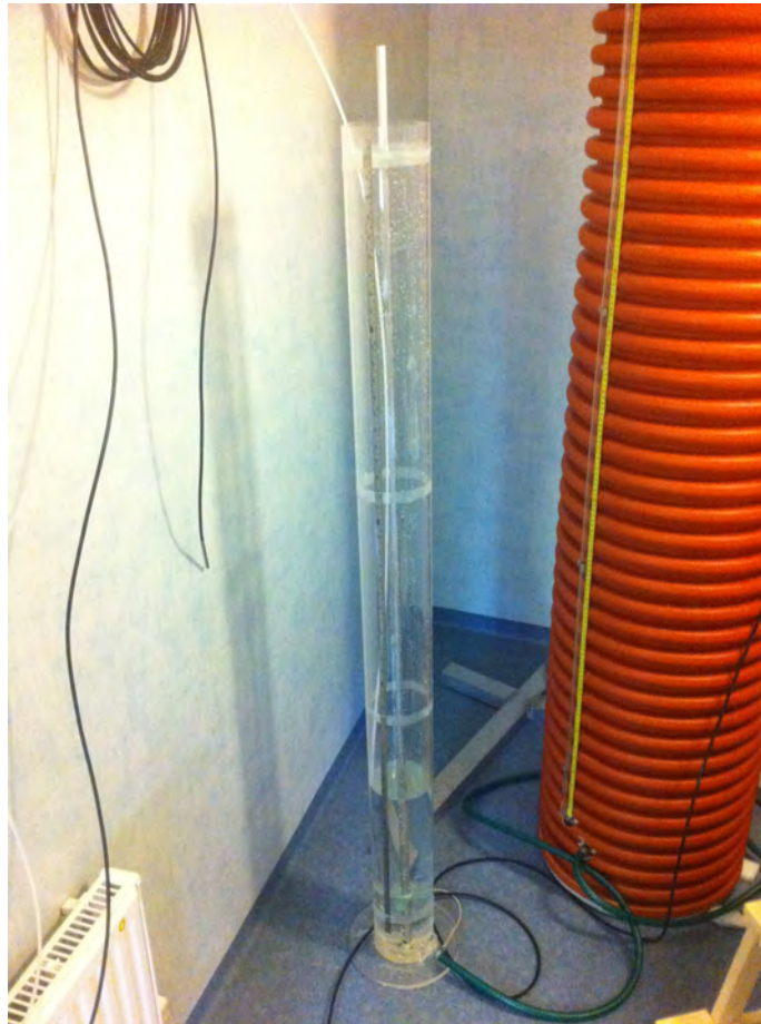
Figure 4.1: The bubbler air hose placed in a plexi glas tube. The red tube used for the radar measurement can be seen to the right.
