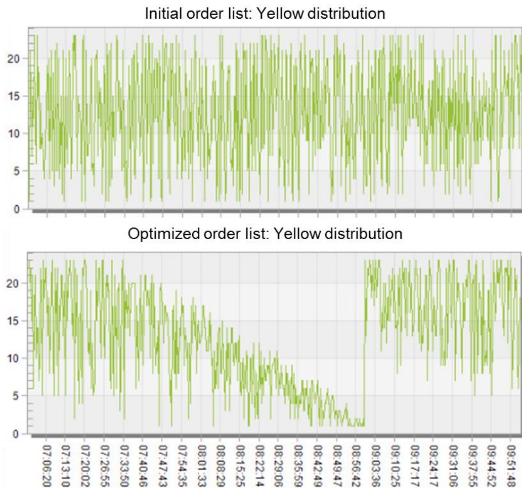
Figure 28: Example graphs illustrating the color distribution of yellow balls over the production time
