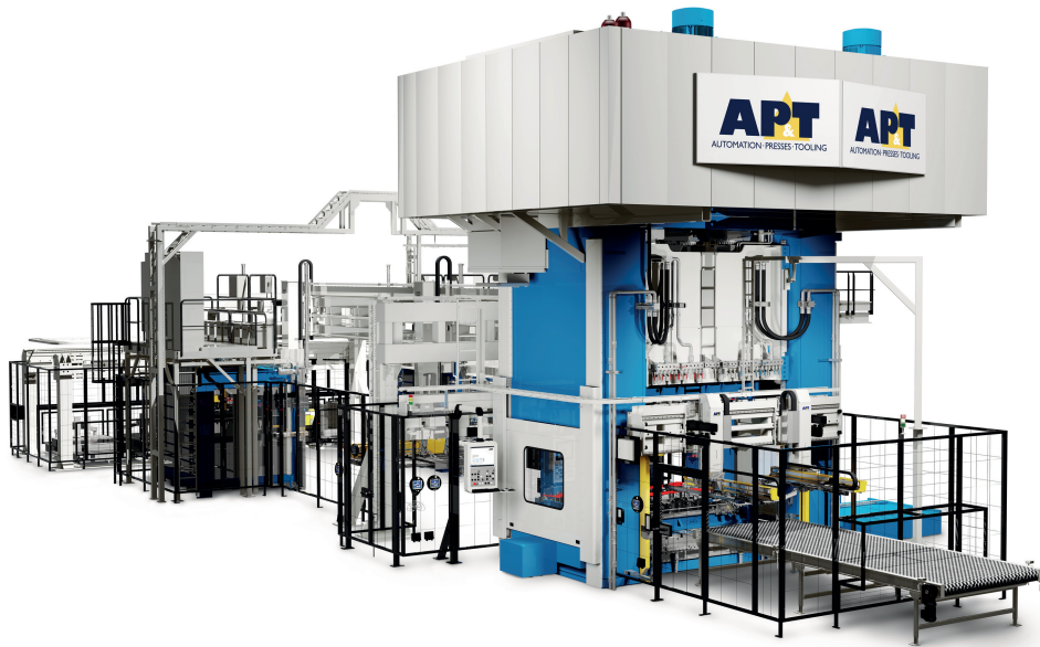
Figure 1.1: Example of press hardening production line sold by AP&T.
