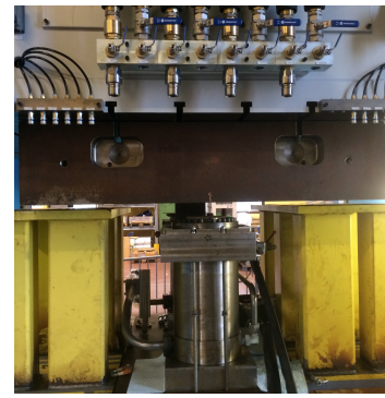
(c) The slide is almost down at the distances and the data collection stops.
