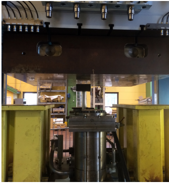
(a) The slide free falls until this position. From this position the slide hold 90 mm/s.
