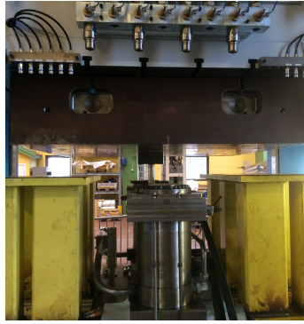
(b) The slide pushing the cylinder connected to the hydraulic outlet down and the data collection starts.
