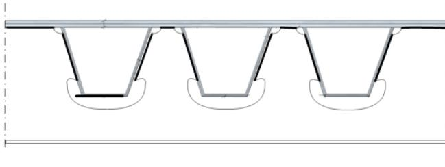
Figure 3. Cross section of conventional orthotropic steel deck [5].
