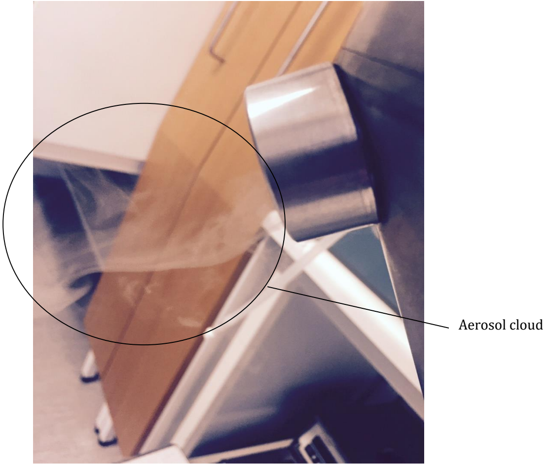
Figure 17. Aerosol cloud (looking like smoke) exiting the rodent outlet.
