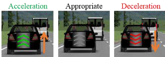
Fig. 2. PRE3 indication at the rear-end of preceding vehicle
