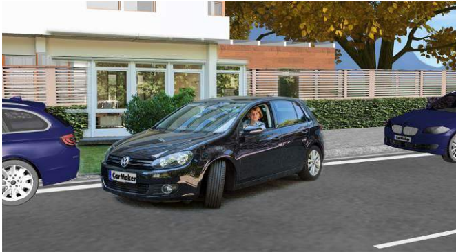
Figure 3: The VIL principle: a real-world test vehicle in a virtual environment, in this case used for testing a parking assist system
