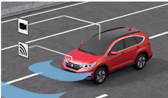
Fig. 3. Sensors used by i-ACC: The camera is located behind the windscreen. The radar sensor is mounted behind the grill.
