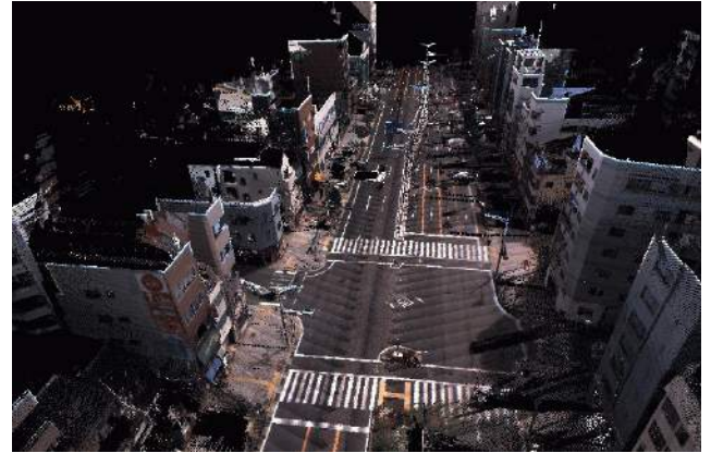
Fig. 1. High density point cloud map measured by MMS
