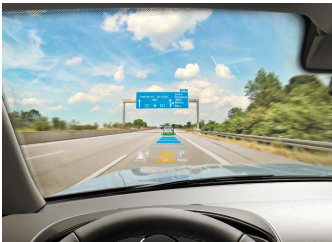
Figure 6: Augmented-Reality HUD with information about the ACC function (source: Continental AG)
