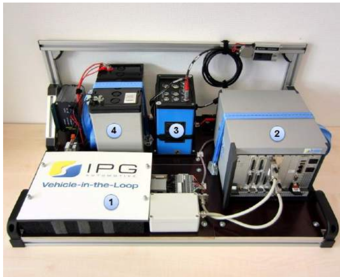
Figure 7: VIL system for a parking assist system, 1 = PDC sensor box, 2 = RoadBox (real-time computer), 3 = INS, 4 = Battery
