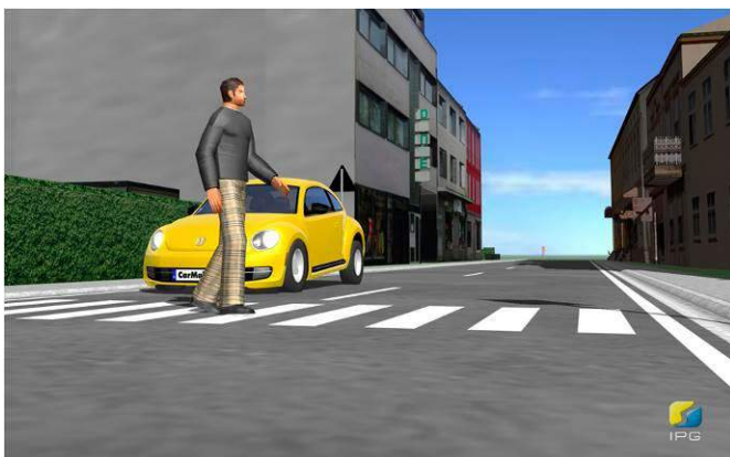
Figure 1: Simulated scenario for testing emergency braking assist systems in IPGMovie
