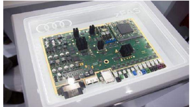
Fig. 4. Compact and in one place: The central driver assistance control unit from Audi is currently the size of a compact laptop – and is set to become even smaller.
