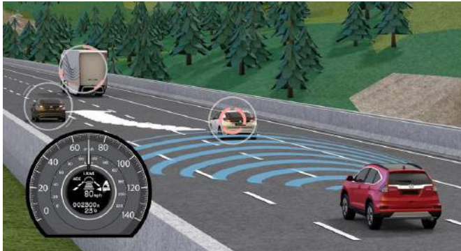
Fig. 4. Cut-in prediction: i-ACC senses all vehicles in front of the ego vehicle, informs the driver about a predicted cut-in and reacts on it.
