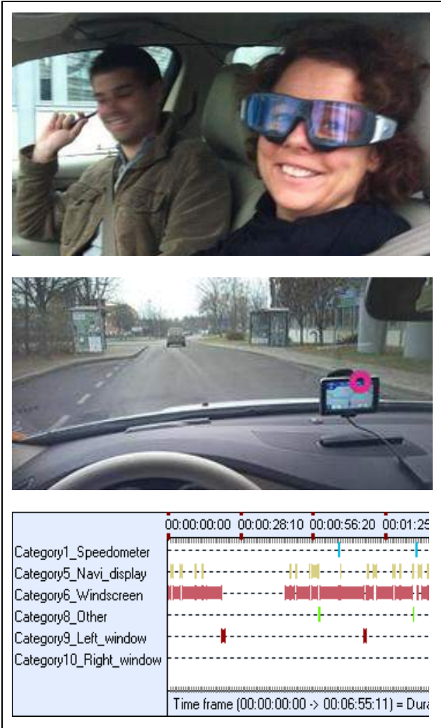
Fig. 3 Eye tracking on road with SMI ETG glasses
