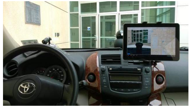
Fig. 1. Mount a Samsung tablet within a car, and use the App MobileUTDrive for data collection.
