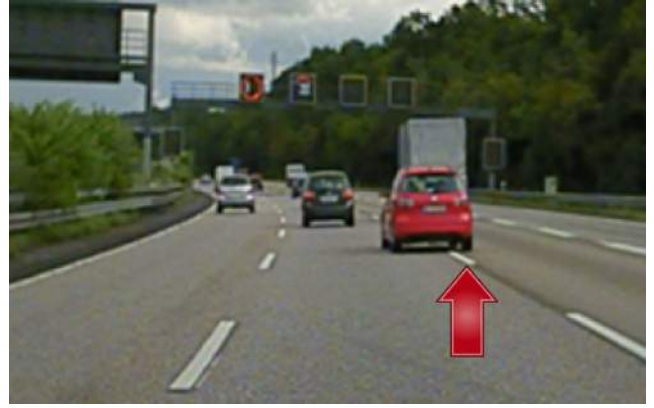
Fig. 8. Ground-truth reference point: Manually annotated point in time for a cut-in, when the right tire touches the lane marking, see red arrow.
