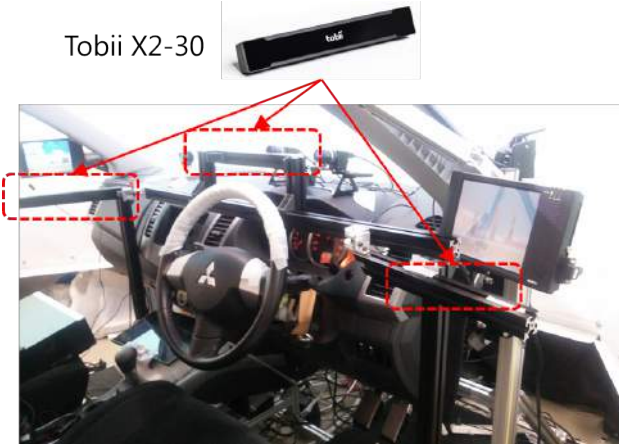
Fig. 4. Snapshot of the driving simulator equipments. Three eye-tracking device, Tobii X2-30 are placed on around the driving seat.
