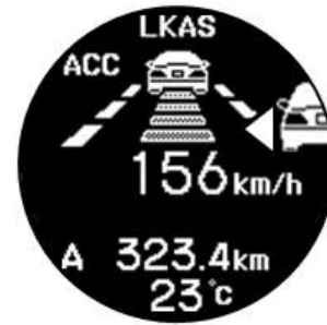
Fig. 5. Display in the cluster instrument showing the cut-in icon on the right side.
