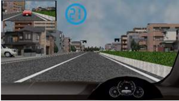
Fig.3. Design of CDT: Indication of remaining green time
