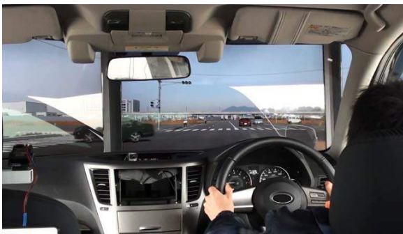
Fig. 3. Frontal view with virtual traffic participants (cars in opposite lane) while driving the instrumented vehicle.
