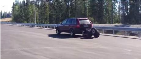
Fig. 11. Friction measurements on the high-speed area.
