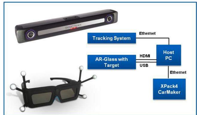
Figure 8: Integration of AR visualization into the test concept
