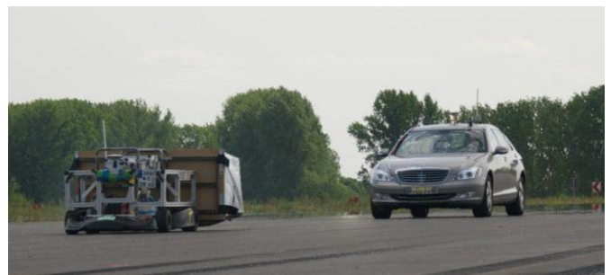
Figure 2: Test method for emergency braking assist systems with dummy targets [2]
