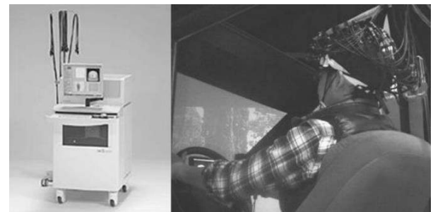
Fig. 6 Multichannel Functional Near-Infrared Spectroscopy and Image of an Experiment
