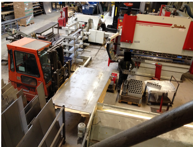
Figure 5.8: Lack of space between the new press brake and the shearing machine.
