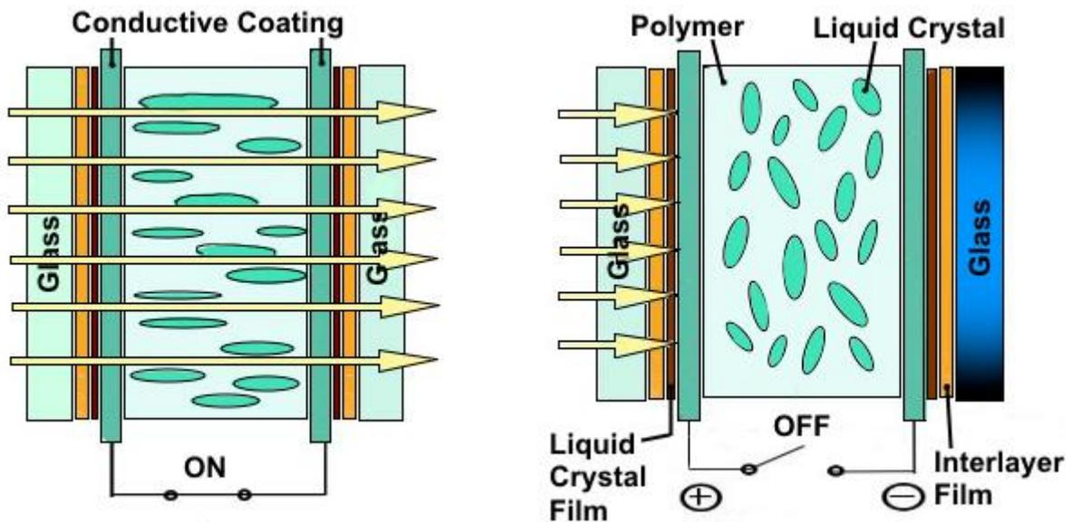
Figure 1 – Polymer Dispersed Liquid Crystal [8]
