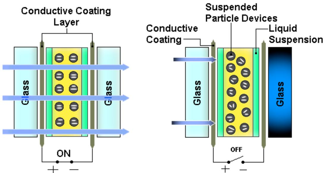
Figure 3 – Suspended Particle Devices [15]
