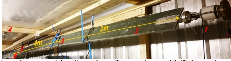
Figure 8: Experimental setup containing (1) transducer, (2) composite material, (3) first accelerometer, (4) thermometer for surrounding temperature, (5) thermometer for material temperature, (6) second accelerometer.
