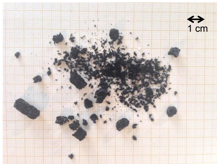
Figure 4. Pellets extracted after 25 minutes of char gasification at 840°C and a steam concentration of 72% (same conditions as for experiment 9).
