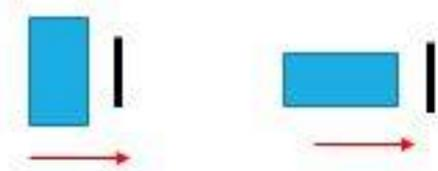
Figure 30: Schematic drawing of probe's positioning: parallel to the length of the notch (left), perpendicular to the length of the notch (right).
