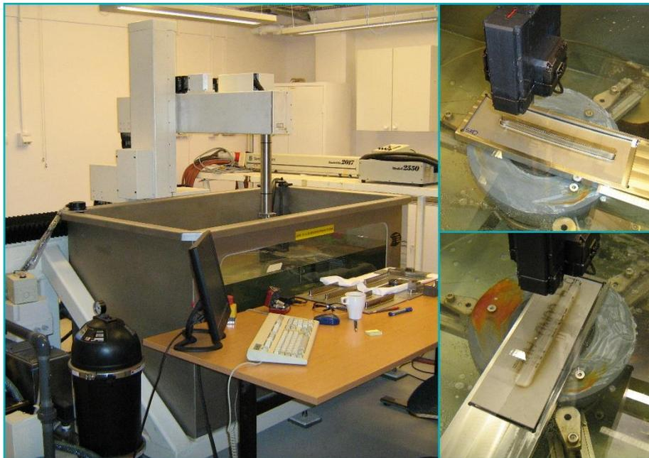
Figure 20: Ultrasonic immersion equipment ScanMaster LS-200.
