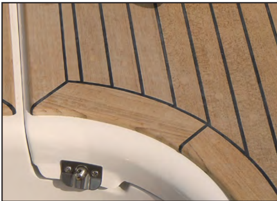
Caulk Teak Deck
