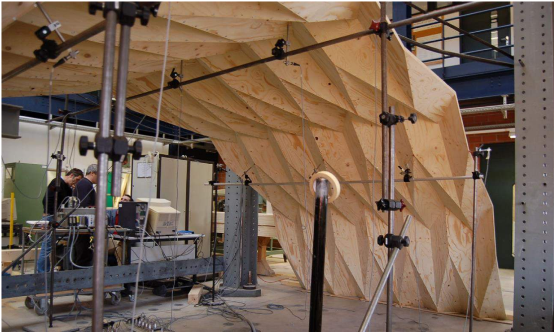
Figure 2.17 A full-scale test of folded plate structure (Buri, 2010).
