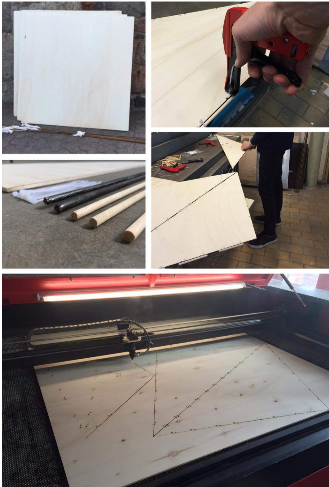
Figure 4.54 Material, laser cutting and mounting of the full scale structure.
