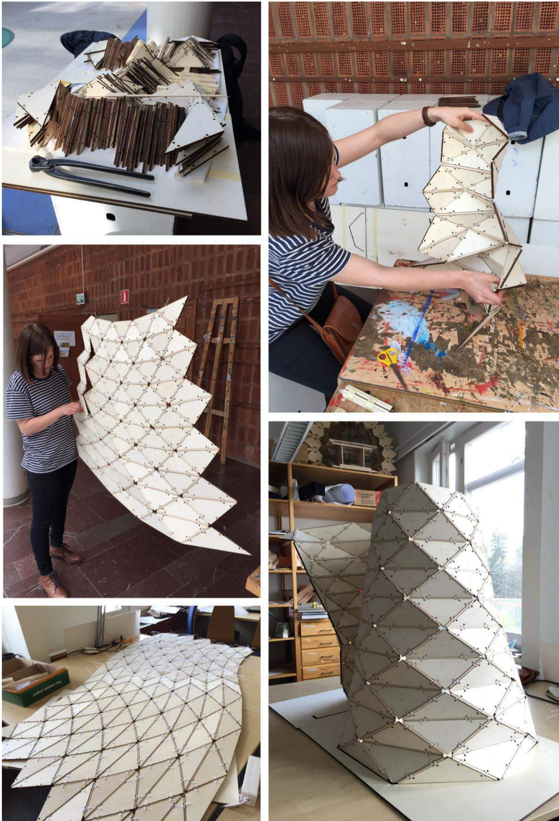
Figure 4.21 Production process, model without stiffening edge bars.
