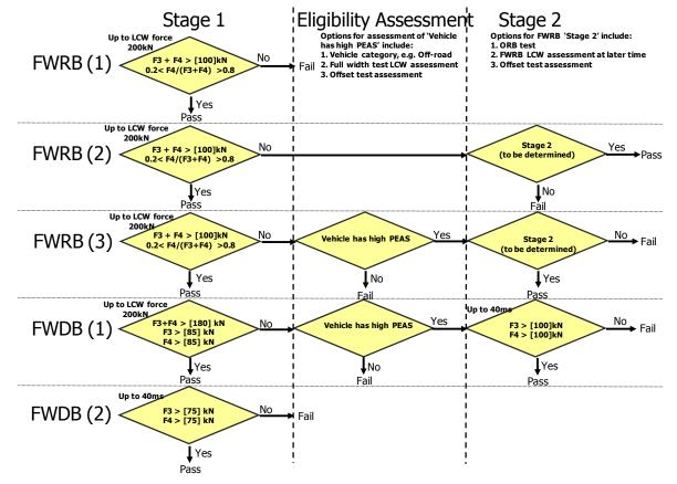
Figure 11. Draft metrics for the FWRB and the FWDB test procedures.
