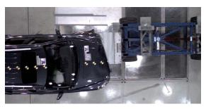
Figure 20. MPDB test with Heavy Vehicle.
