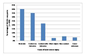
Figure 3. Cause of most severe injury for belted MAIS 2+ occupants in CCIS data set (Note: a small number of occupants are counted twice as they have two most severe injuries by more than one cause).
