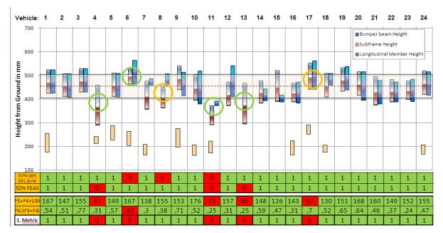
Figure 10. Geometry of longitudinal member, bumper beam and subframe height, geometrical assessment according to US voluntary commitment and FWRB metric assessment for 24 different vehicles.
