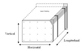
Figure 15. Barrier axis definition.
