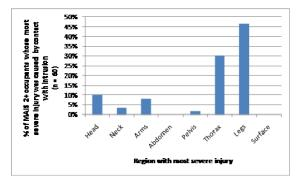
Figure 4. Distribution of 'most severe' injury by body region for MAIS 2+ belted occupants with their most severe injury caused by contact with intrusion.
