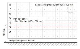
Figure 8. Overview of the specifications of the LCW (rows, columns, height of ground, Part 581 zone).
