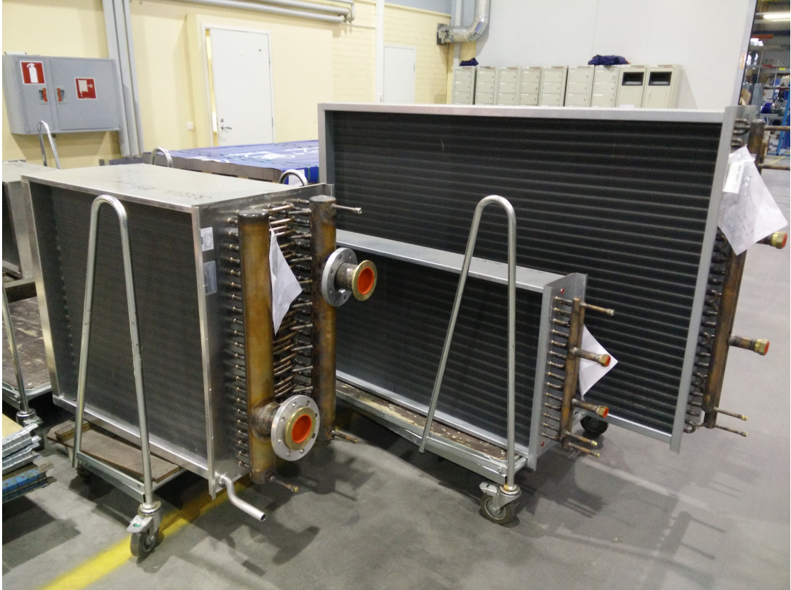
Figure 1.1: Different sizes of fin-and-tube heat exchangers are designed for different applications
