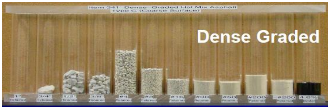
Figure 6: Dense graded asphalt mix (Way, George, 2012)
