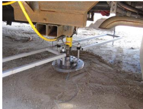
Figure 18: Hydraulic Jack for plate bearing capacity measurement (Iowa State University, 2015)
