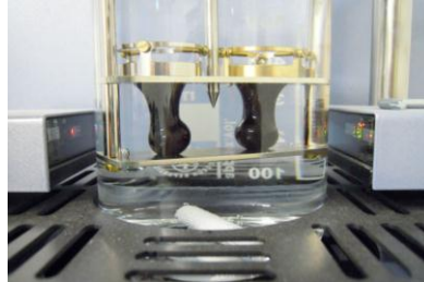
Figure 14: Ring and Ball method (Bieder & Jenzer , 2011)
