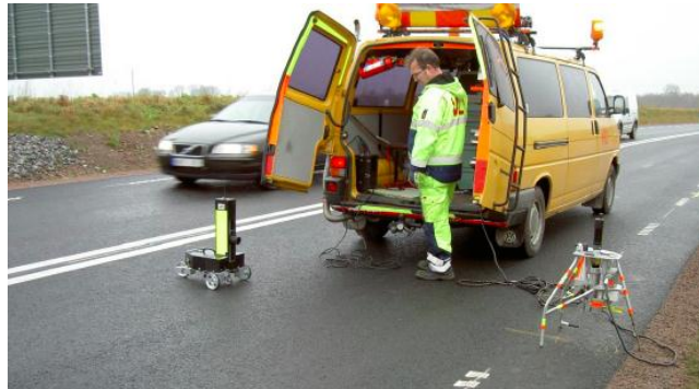
Figure 25: Profile cross section measurement with Primal (Karlsson, 2015)
