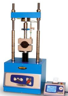
Figure 15: Marshall/ CBR Compression (Matest, n.d.)
