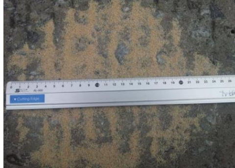
Figure 22: Sand Patch Test (Kim, et al., 2013)
