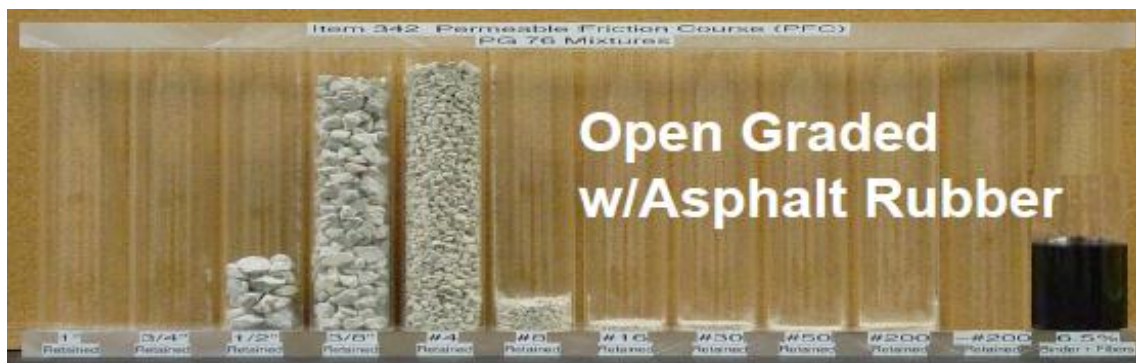
Figure 7: Aggregate content in open graded asphalt mix (Way, George, 2012)
