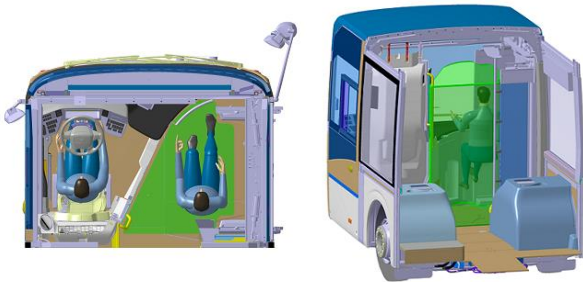
Figure 5: Available design space in the bus. Top view to the left, rear view to the right.
