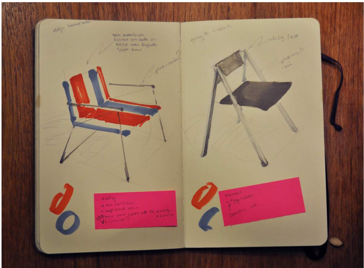
Figure 58. Hinge five with redifined proportions & Concept A - a combination of hinging and sliding techniques.
