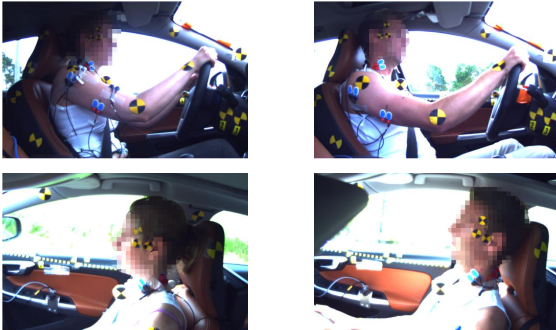
Figure 4. Pictures of one female (left) and one male (right) volunteer in the driver (top) and passenger (bottom) position during initial braking with a motorized seatbelt (~250 ms after belt pretension).
