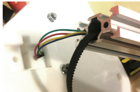
FIGURE 5.9: y stepper cables led through the V-Slot
