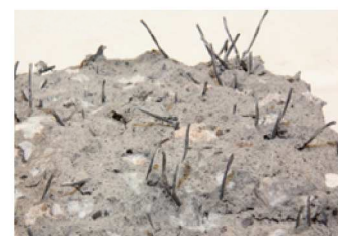
Figure 15 MiniBars in different materials; a) AR-glass MiniBars, and b) basalt MiniBars.
