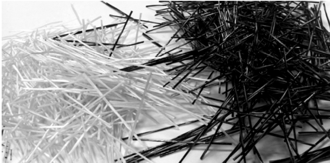
Figure 15 MiniBars in different materials; a) AR-glass MiniBars, and b) basalt MiniBars.
