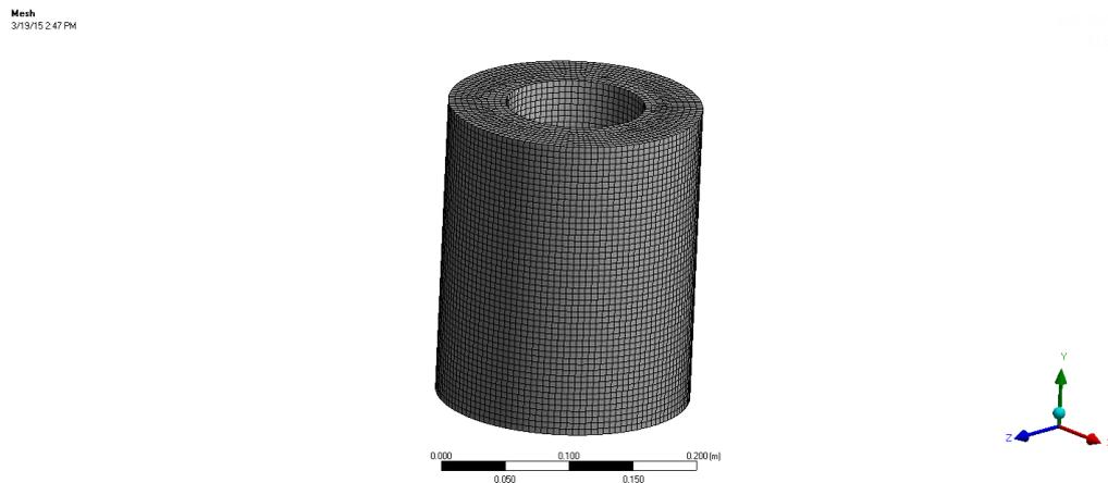
Figure A8.3 – The mesh size used for the rubber spring.
