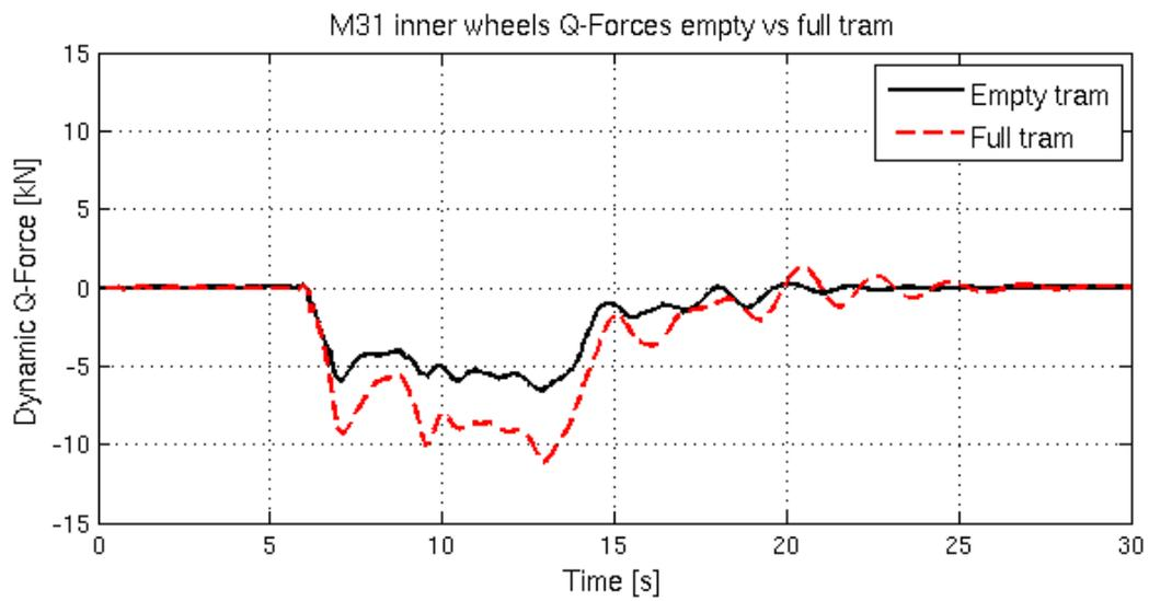
Figure 5.14 – Comparison between  $Q$ -forces obtained during simulations with M31 model. The black lines represent an empty tram and the dashed red lines a fully loaded tram. Top figure shows the  $Q$ -forces on the outer wheels and bottom figure shows the  $Q$ -forces on the inner wheels.
