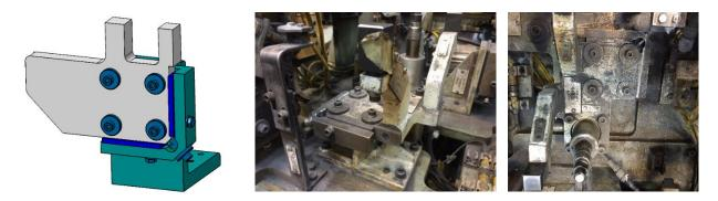
Fig. 3. (a) 3D model of a shimming plates and fixture part; (b) Fixture application at Olofström plant of VCC
