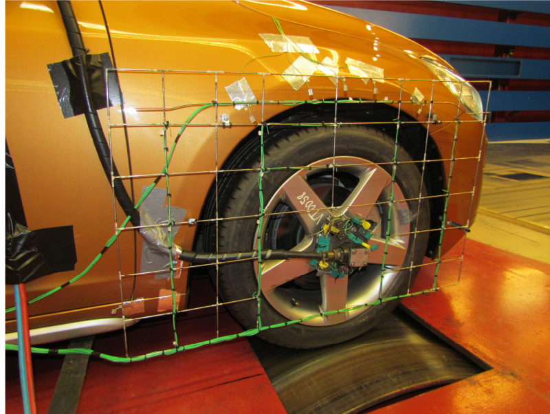
Figure 18. Brake cooling test setup
