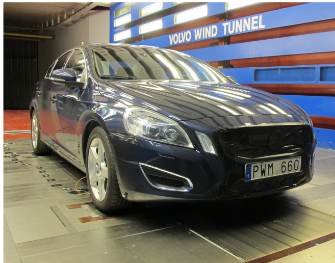
Figure 17. Overview of the test setup and covered cooling flow inlets
