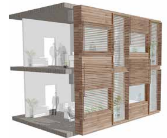
2. External sliding panels (movable)
