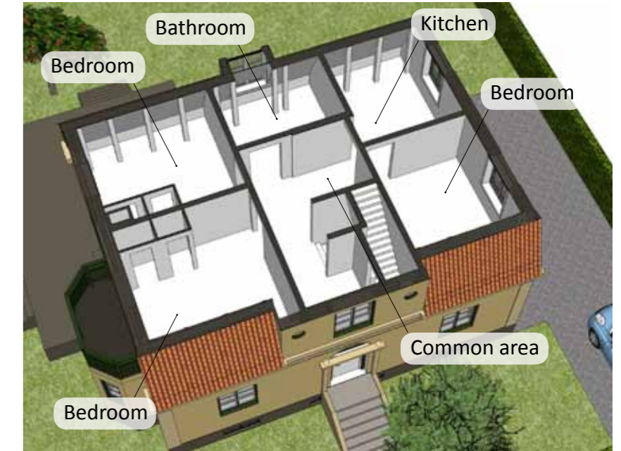
Fig. 39. Cut of the plan in the upper floor, a proper kitchen installed, bigger common areas and smaller bathroom.
