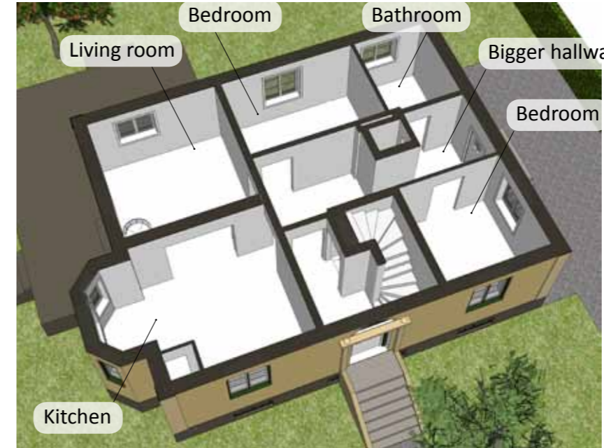
Fig. 38. Cut of the plan in ground floor, kitchen moved, 1 bedroom added and bigger hallway.
