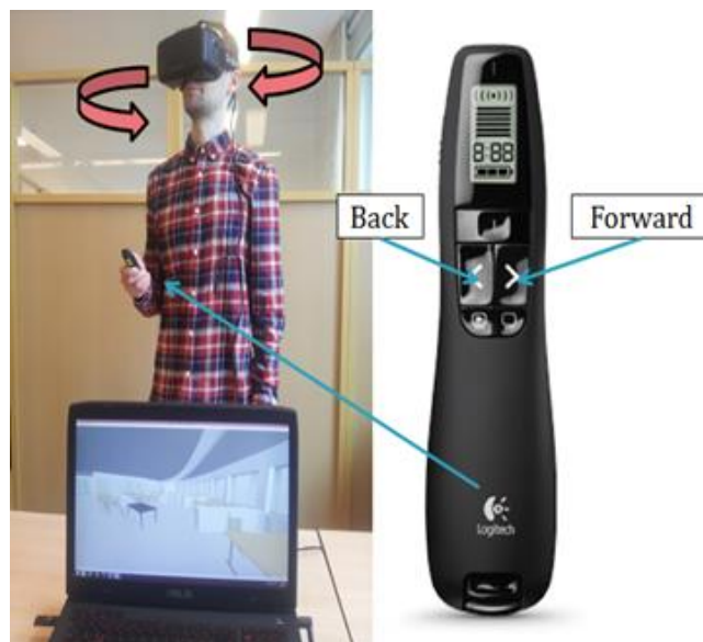
Figure 7 Technical system required to navigate virtually
