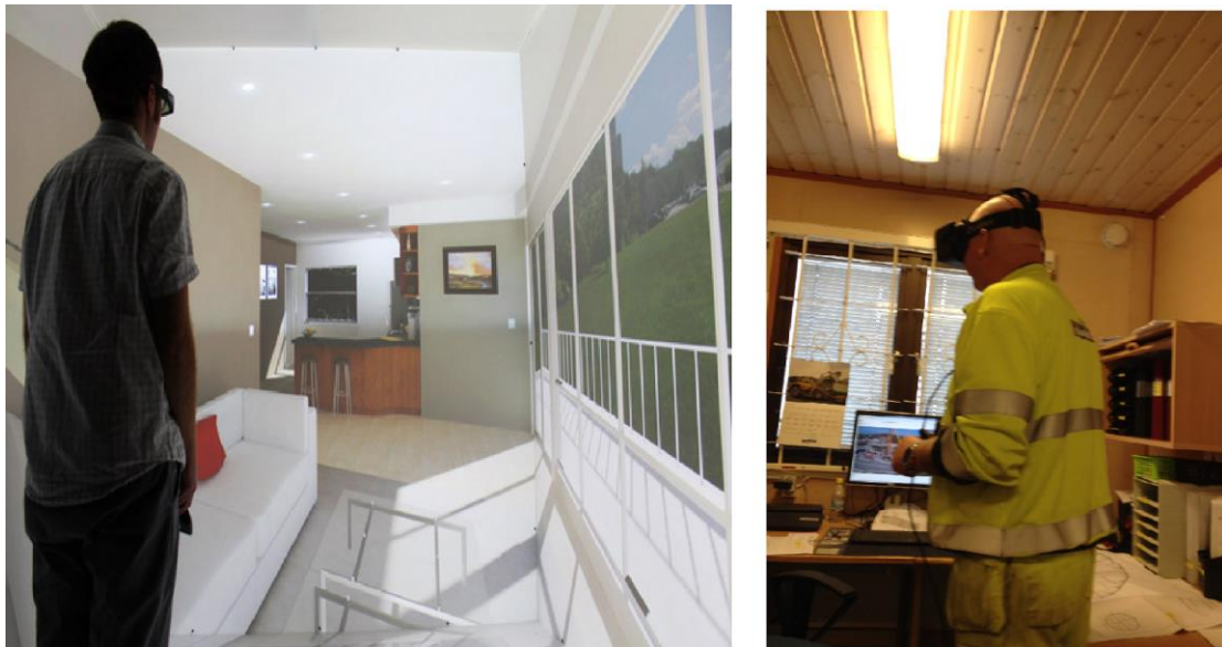
Figure 4 Immersive visualisation using a CAVE system (left) vs. a Head Mounted Display (Right)
