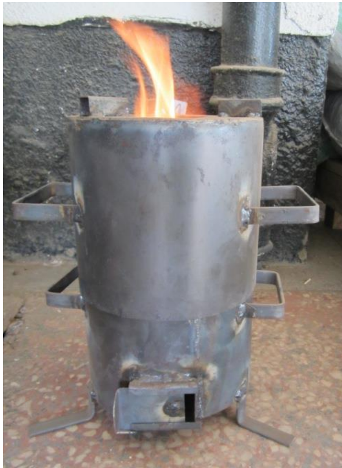
Figure 10 Jiko Makini. A picture of the gasification stove Jiko Makini (Narayan, 2012).
